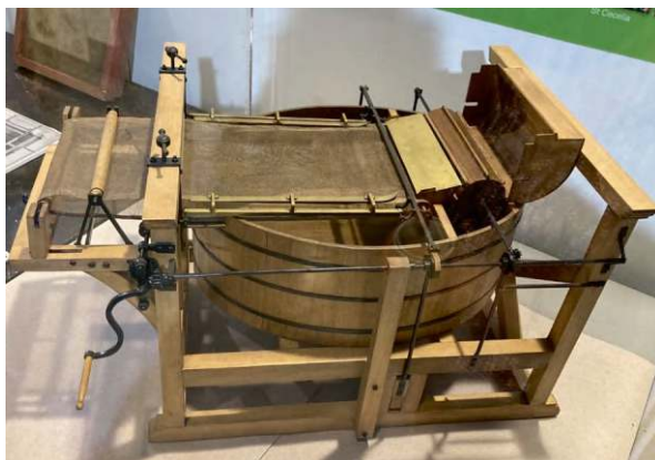
Fig. 3.8 First model of the papermaking machine invented by N.-L. Robert. https://www.worldhistory.org/image/17305/papermaking-machine/
