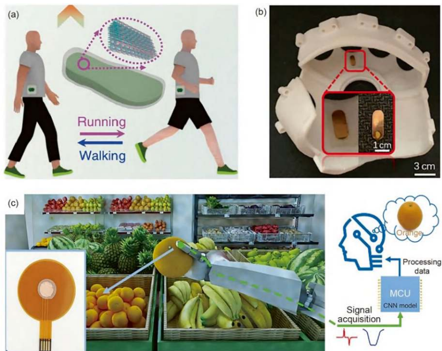
Fig. 1.6 User identification and object recognition. (a) Smart wearable systems for human motion monitoring and remote emergency rescue; (b) smart gloves with haptic feedback; (c) object recognition by a robotic gripper equipped with dual-mode tactile sensors. (a) Reprinted from (Dong K et al., 2020), Published 2020 by Springer Nature with open access. (b) Reprinted from (Zhu et al., 2020). Published 2020 by AAAS with open access. (c) Reprinted with permission from (Li et al., 2021), Copyright 2020: Elsevier
