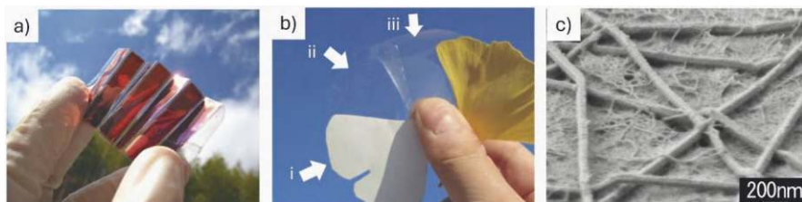
Fig. 12.11 Solar cell devices: (a) Photograph of the foldable and lightweight paper solar cell produced using the transparent conductive nanopaper; (b) photograph of cellulose (i) traditional write paper, (ii) transparent nanofiber paper, and (iii) transparent conductive nanofiber paper; and (c) scanning electron microscopy image of the transparent conductive nanofiber paper, where it is possible to observe the silver nanowires entangled with the cellulose nanofibers. Adapted from Nogi et al. (2015). Published 2015 by Nature Portfolio under the terms of the Creative Commons CC BY4.0
