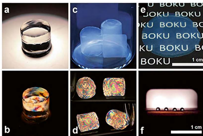
Fig. 19.2 Visualized appearance and properties of CNF alcogels (a, b) obtained from an aqueous dispersion of 2-CC ( 9.5 \text{ mg mL}^{-1} ) by acid-induced gelation and solvent exchange. Immersion in a solution of PMMA in acetone and consecutive \text{scCO}_2 antisolvent precipitation and \text{scCO}_2 drying in a single batch afforded CNF/PMMA composite aerogels (c–f; \rho_B = 14.8 \text{ mg cm}^{-3} ) with conformal ultrathin PMMA coating (c). Birefringence patterns under crossed polarizers confirmed preservation of nematic orientation throughout all conducted manipulations (b, d). The obtained materials were transparent (e, thickness 2 mm) and hydrophobic (water contact angle of 119.4^\circ \pm 7.5^\circ ) as seen from the shape of four water droplets resting on an aerogel disc illuminated by a light source (f). (Reprinted with permission from Plappert et al. (2018). Copyright 2018 American Chemical Society)
