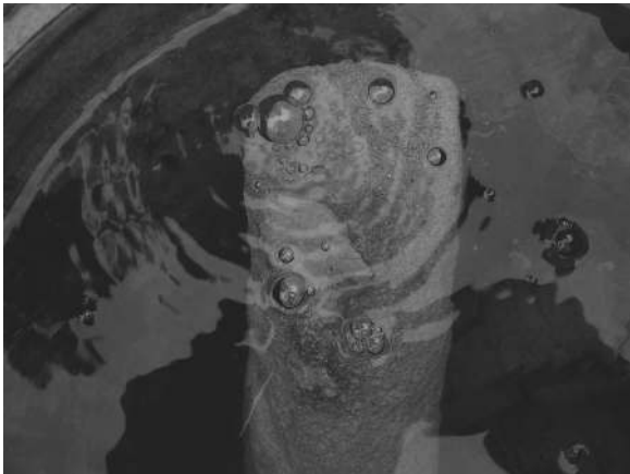
FIGURE 1.19 Air bubbles from the immersed dry weak sandstone sample collected from the proposed site for the construction of a coal handling plant (CHP), Northern Coalfields Limited, Gorbi, Madhya Pradesh, India. [After Sanjay Kumar Shukla, Subsoil Investigation for the Estimation of Load-Bearing Capacity of Foundation Soil at the Proposed Site for the Construction of a Coal Handling Plant (CHP), Northern Coalfields Limited, Gorbi, MP, India. A technical report dated 16 October 2006, Department of Civil Engineering, Institute of Technology, Banaras Hindu University, Varanasi, India, 2006.]
