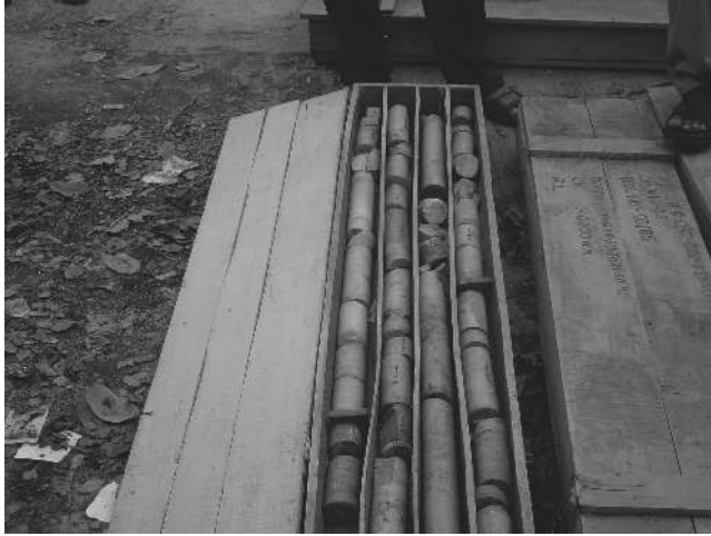
FIGURE 1.22 Rock cores in a core box.
