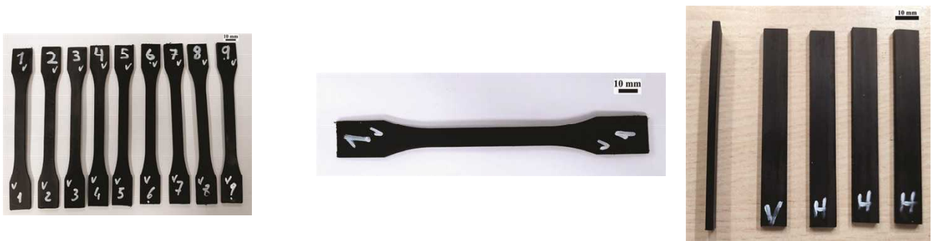
Figure 5. Machined specimens for tensile (left) and flexural tests (right).
