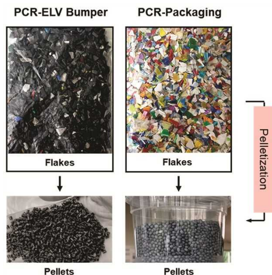
Figure 1. Optical appearance of flakes before compounding and pellets after compounding for PCR-Packaging and PCR-ELV-Bumper materials.
