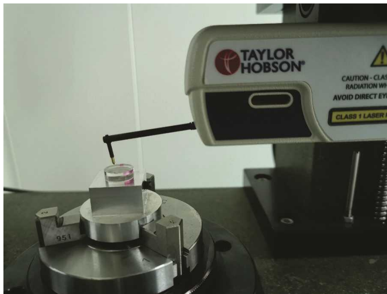
Figure 2. Setup of PMMA workpiece measurement with a Taylor Hobson device.
