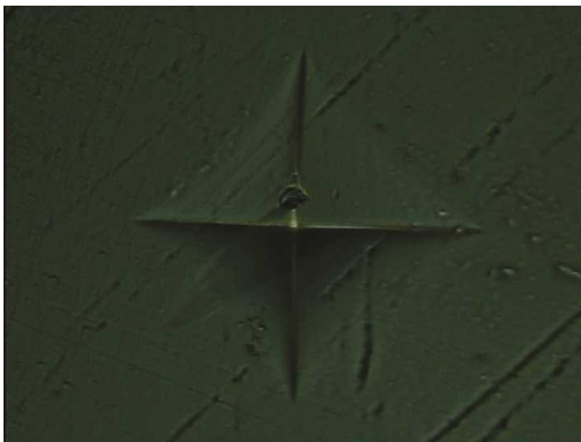
Figure 7. One typical indentation point of cryogenically cooled PMMA under a microscope.
