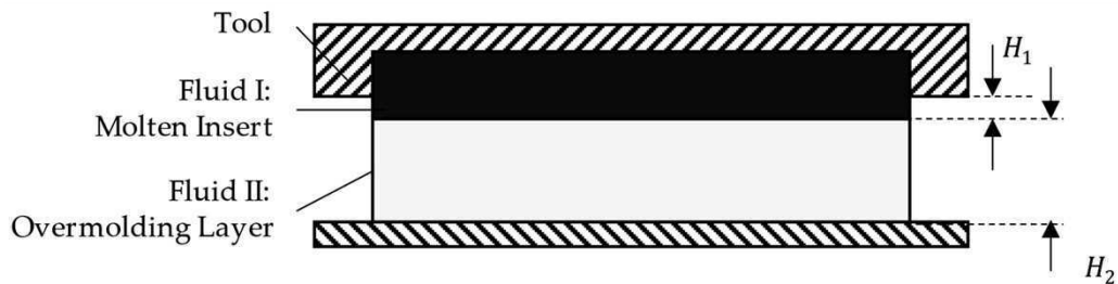
Figure 9. Schematic representation of an overmolding setup with an overmolding layer and an insert, where part of the insert height is covered by a tool.
