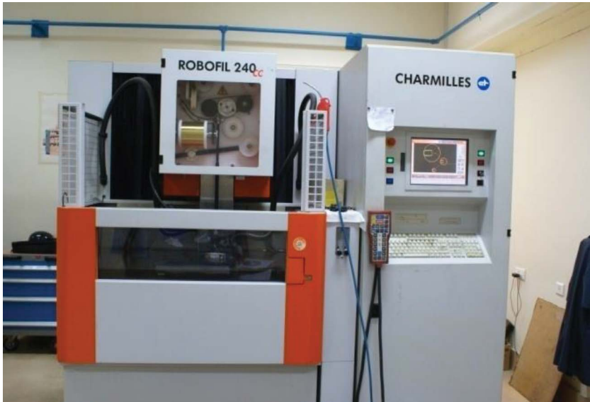
FIGURE 4.2 ROBOFIL 240CC WEDM setup.
