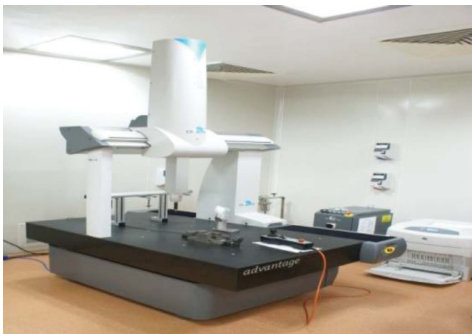
FIGURE 4.3 Hexagonal DEA CMM setup.
