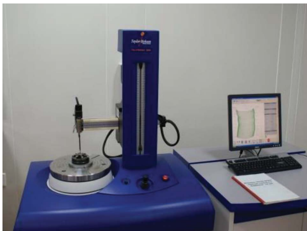
FIGURE 4.5 Taylor Hobson Talyrond 365 used to measure cylindricity.
