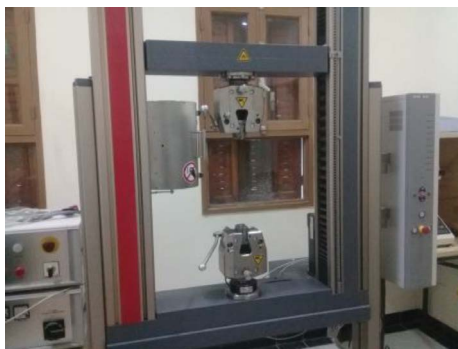
FIGURE 6.5 View of the tensile machine used in this study.
