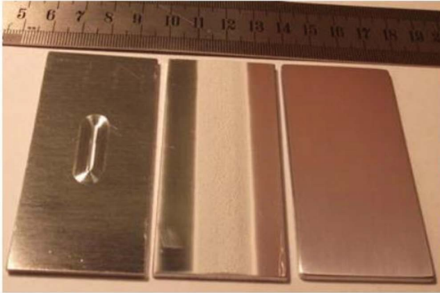
FIGURE 2.15 The repair process of damaged Al part with CS technology (Yandouzi et al. 2014).
