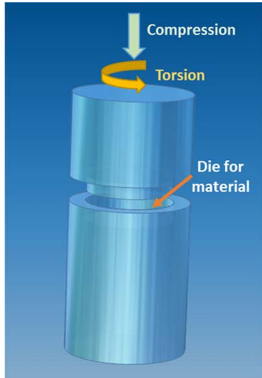
FIGURE 5.10 Schematic layout of high-pressure torsion process.
