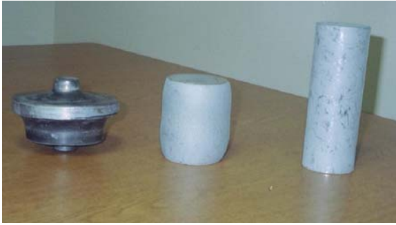
FIGURE 11.5 Results obtained for the preform and final stages. Used with permission from Gunasekera, J.S., Mayer, R., Al-Mufadi, F., 2005. Case Study: Optimization of Forging a Rotating Part Using Computer Modeling at Queen City Forging Co. Cincinnati, OH.
