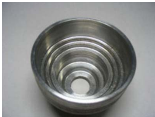
FIGURE 3.2 Digital camera barrel made of AZ31B alloy by hot extrusion. Reused with permission from Park, C.W., Kim, Y.H., 2012. A study on the manufacturing of digital camera barrel using magnesium alloy. International Journal of Precision Engineering and Manufacturing 13, 1047–1052. https://doi.org/10.1007/s12541-012-0136-x ; springer.
