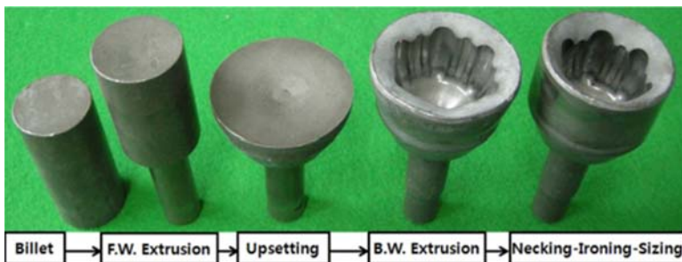
FIGURE 3.3 Fabrication of outer race using multistage cold forging process. Reused with permission from Ku, T.-W., Kang, B.-S., 2014. Tool design and experimental verification for multistage cold forging process of the outer race. International Journal of Precision Engineering and Manufacturing 15, 1995–2004. https://doi.org/10.1007/s12541-014-0556-x ; Springer.
