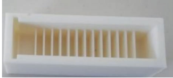
Fig. 7 3D Printed mould for artificial muscle
