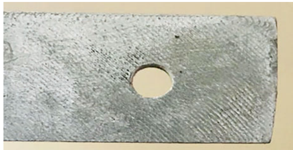
Fig. 4 Injection moulded slit of ABS-15% Al
