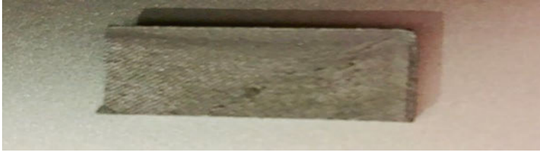
Fig. 4 Injection moulded slit of ABS-15% Al
