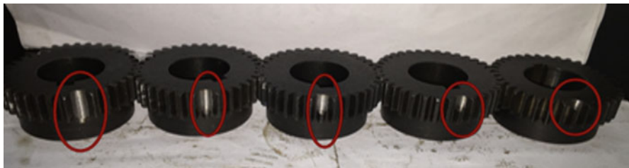
Fig. 2.5 Five kinds of gears with different degrees of broken teeth (the width of the broken teeth is 1/5, 2/5, 3/5, 4/5, 1 of the tooth width, respectively)
