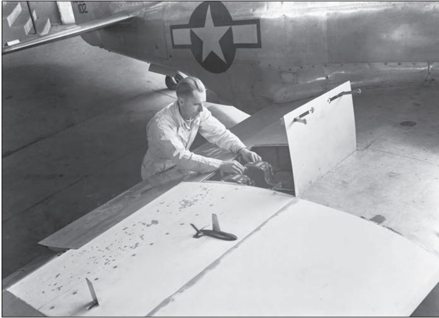
Figure 11.37 Photograph of a test model mounted on the wing of the P-51 used for the NACA Wing-Flow transonic tests, circa 1946. (NASA).
