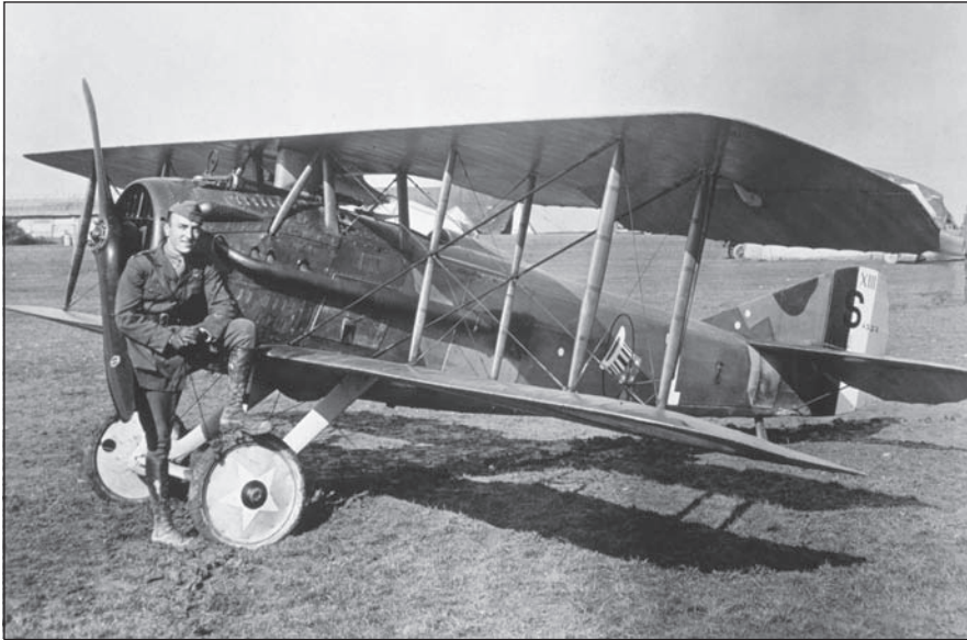
Figure 3.50 The French SPAD XIII, an example of a strut-and-wire biplane from World War I. Captain Eddie Rickenbacker is shown at the front of the airplane. (© MPI/Stringer/Getty Images).
