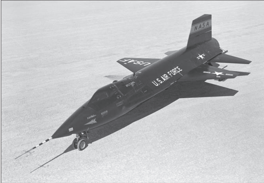
Figure 9.18 The X-15 hypersonic research vehicle. Designed and built during the late 1950s, it served as a test vehicle for the U.S. Air Force and NASA. (NASA).
