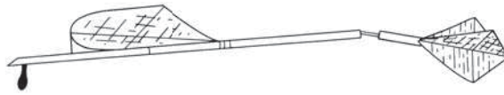
Figure 4.59 The first modern configuration airplane in history: George Cayley's model glider of 1804.
