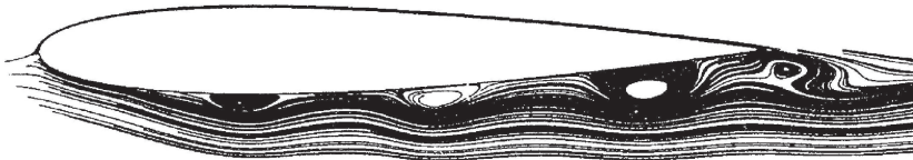
Figure 20.14 Streamline pattern over the bottom of an NACA 0012 airfoil, over which a series of jets is distributed which are alternatively blowing or sucking mass into or out of the flow, with the overall net mass injected into the flow being zero—a zero-mass jet array. (Data Source: Hassan, A. A., and JanakiRam, R. D.: “Effects of Zero-Mass ‘Synthetic’ Jets on the Aerodynamics of the NACA-0012 Airfoil,” AIAA Paper No. 97-2326, 1997).
