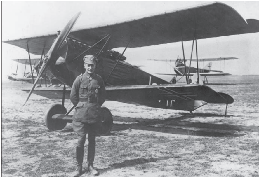
Figure 4.65 The World War I Fokker D-VII, one of the most effective fighters of the war, due in part to its superior aerodynamic performance allowed by a thick airfoil section. (© Chronicle/Alamy).
