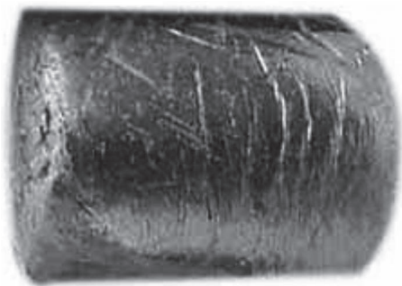
FIGURE 2.5 Plastic wrapped THC as supplied by the refractory manufacturers to iron and steel industries.
