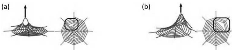
FIGURE 11.2 Geometric and material nonlinearity focuses severe point loads on radial arms of spider web, which leads to localized failures that preserve continuity of the web. (From Cranford 2012].)
