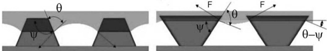
FIGURE 13.7 Cassie state resulting from hydrophobic and hydrophilic wetting with different values of the contact angle \theta and pillar texture angle \psi . (From [Tuteja 2008].)
