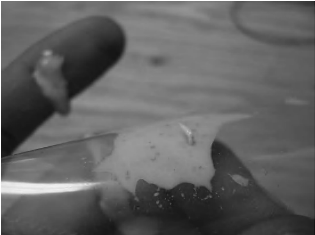
FIGURE 6.9 Plug formed by coagulation with tire inner tube sealant compound.
