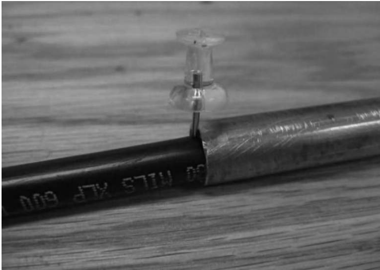
FIGURE 10.3 Self-healing flooding cable for medium-power underground electric power distributions using viscous PIB to seal insulation breaches undergoing puncture test.
