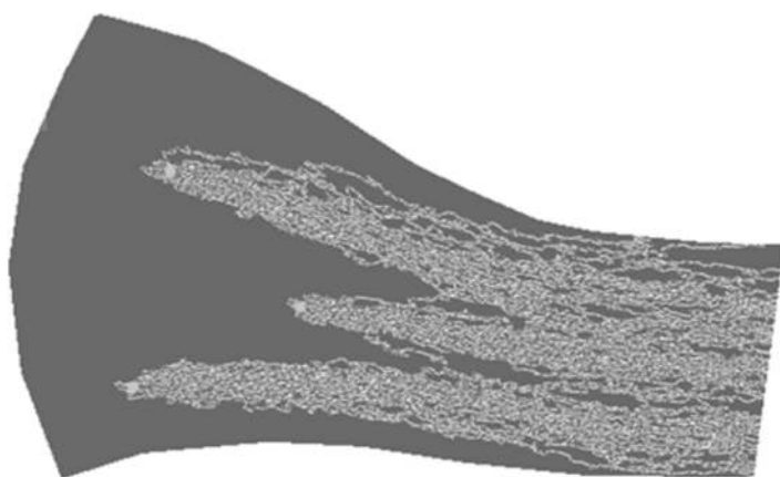
FIGURE 8.16 Contaminant molecules moving with convection and dispersion.
