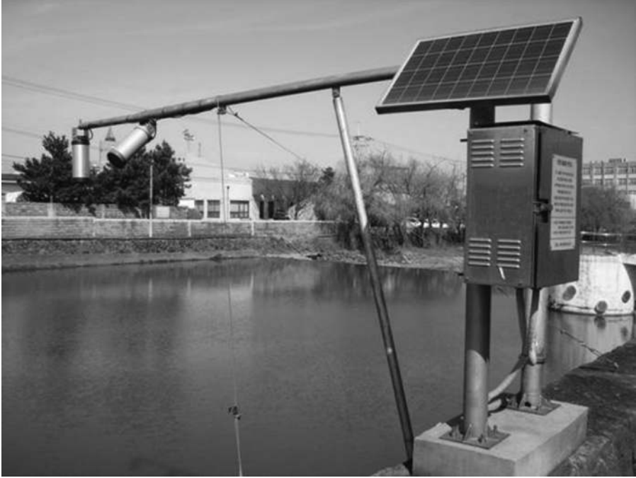
FIGURE 5.11 A sensor used to measure the stream stage.
