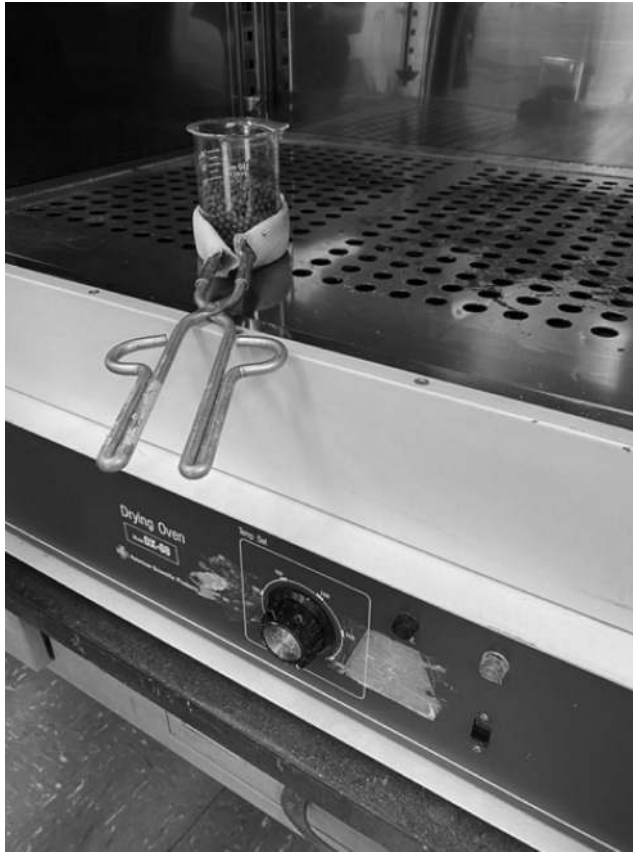
FIGURE 10.4 Oven-drying the sample. (Photograph by the author.)
