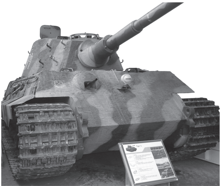
FIGURE 7.7 King Tiger tank of WWII, which used ‘flame-hardened’ steel armour.
