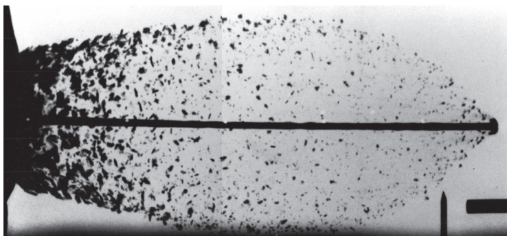
FIGURE 11.7 Shaped-charge jet penetration of armour (courtesy of J Backofen Jr).
