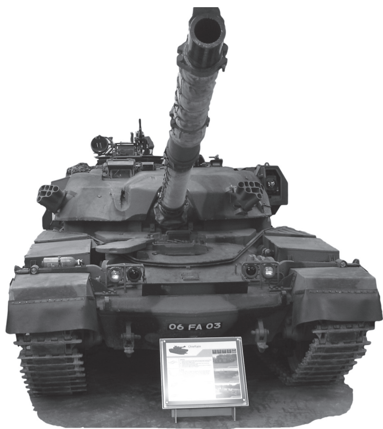
FIGURE 7.2 Chieftain Main Battle Tank (MBT) employing a cast steel turret.
