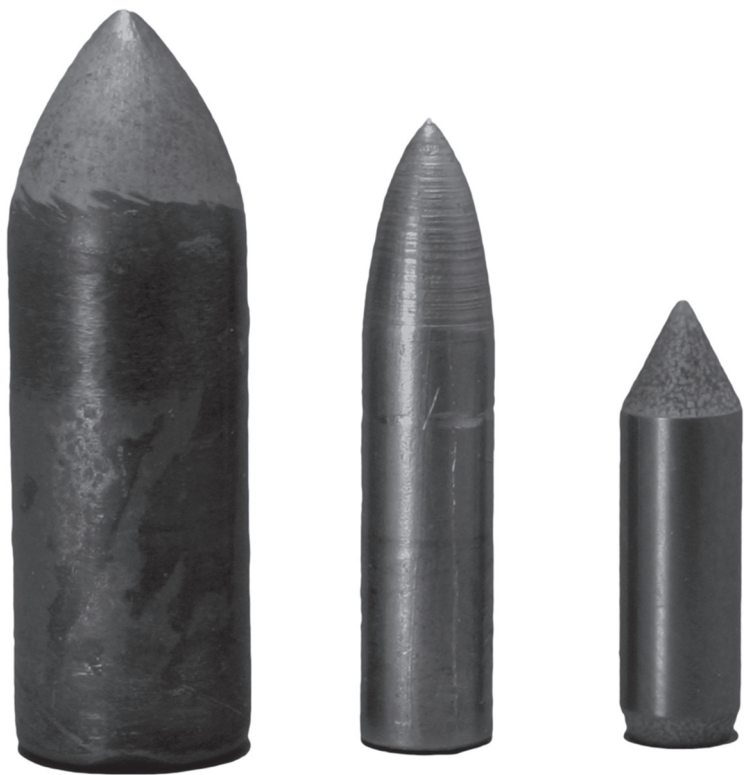
FIGURE 3.4 From left to right: 14.5×114-mm BS41 Armour-Piercing Incendiary (API) core, 7.62×54-mm R B32 API core and 7.62×51-mm Förenade Fabriksverken (FFV) core.
