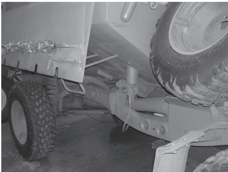
FIGURE 11.10 A South African Buffel showing the V-shaped hull design. The Christmas decorations are not usually part of the camouflage.
