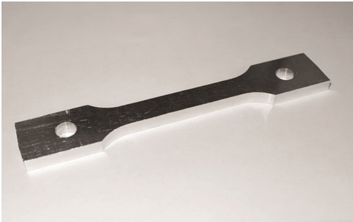
Fig. 1.2 Test specimen machined from a plate that is too thin to give a large enough circular cross section. (Courtesy of Westmoreland Mechanical Testing and Research Inc.)
