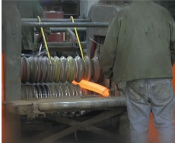
Fig. 5.4 Hot working of a titanium bar (courtesy of TSI Titanium)
