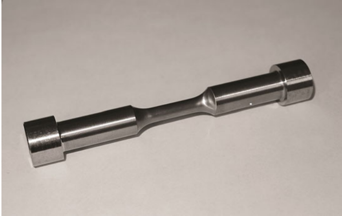
Fig. 1.1 Test specimen machined from a plate thick enough to give a circular cross section. (Courtesy of Westmoreland Mechanical Testing and Research Inc.)
