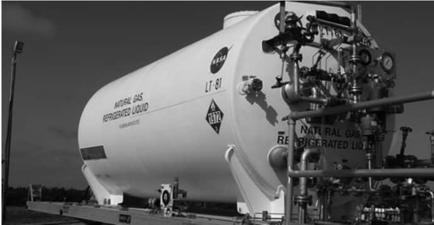
FIGURE 13.20 Liquid natural gas tanker designed and built by AECOM employees to support NASA's Morpheus program. Source: NASA, www.aecom.com/blogs/wp-content/uploads/sites/103/2015/07/LT-81-LNG_690x355.jpg
