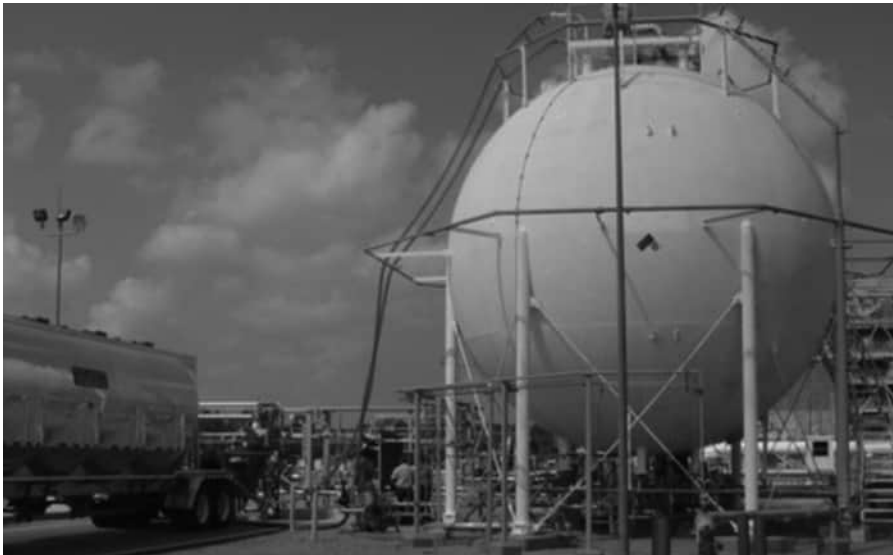
FIGURE 6.21 The 218- \text{m}^3 \text{LH}_2 tank shown with its annulus being filled with glass bubble insulation from an over-the-road pressure differential trailer [44]. Source: NASA
