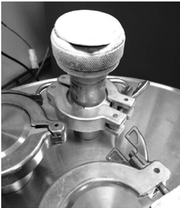
FIGURE 7.6 Vacuum relief device (25-mm lift plate) on a cryostat vacuum chamber. Source: J. Fesmire
