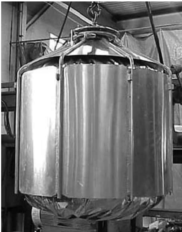
FIGURE 7.13 Aluminum LHe dewar with vapor-cooled thermal shield. Source: Meyer Tool & Mfg.
