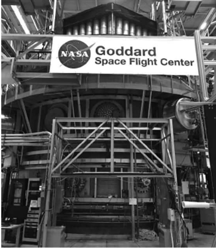
FIGURE 7.18 Vacuum chamber at NASA Goddard Space Flight Center for testing of elements of the James Webb Space Telescope and other spacecraft. One of the cryopumps is shown in the middle right. Source: J. Fesmire
