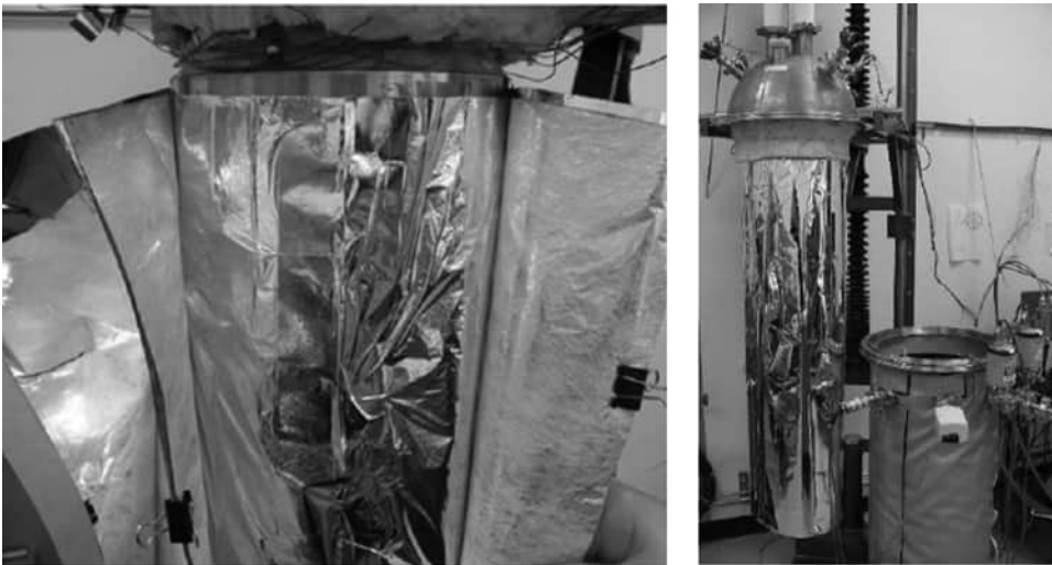
FIGURE 3.3 LEFT: Preparation of MLI test specimens on the Cryostat-100 cold mass assembly: layer joining A134. Right: Completed test specimen A138 for insertion to the vacuum chamber [1].
