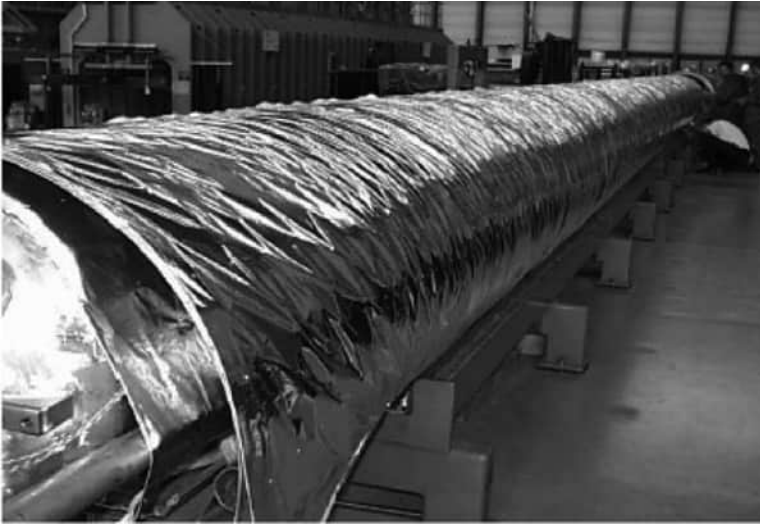
FIGURE 7.9 Prefabricated MLI blankets upon installation.
