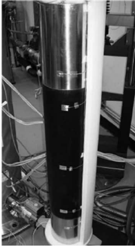
FIGURE 2.24 Installation of a SOFI clamshell test article on the cold mass assembly of thermal conductivity instrument Cryostat-100.
