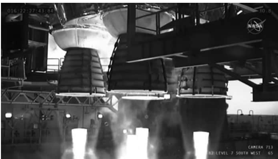
FIGURE 13.17 The core stage for the first flight of NASA's Space Launch System rocket is seen in the B-2 Test Stand during a hot fire test January 16, 2021, at NASA's Stennis Space Center near Bay St. Louis, Mississippi. Source: NASA ( Television )
