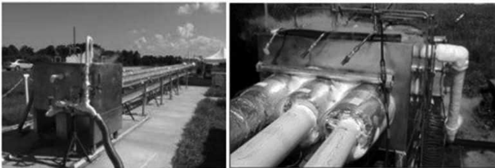
FIGURE 6.13 Simplified diagnostic chart of the cryogenic pipeline test apparatus. Thermal guard boxes at the ends of a pipe under test are used to make the fluid connections and for temperature control [32].
