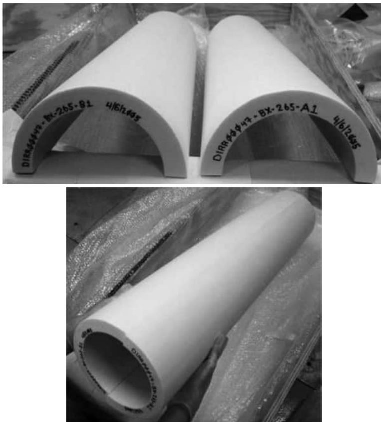
FIGURE 2.23 One of five 1-m-long cylindrical clamshell test articles were produced for testing using a cylindrical thermal conductivity test instrument (Cryostat-100). Machined thickness of approximately 25 mm is shown in the left view, while the precise longitudinal fit-up is shown in the right view.
