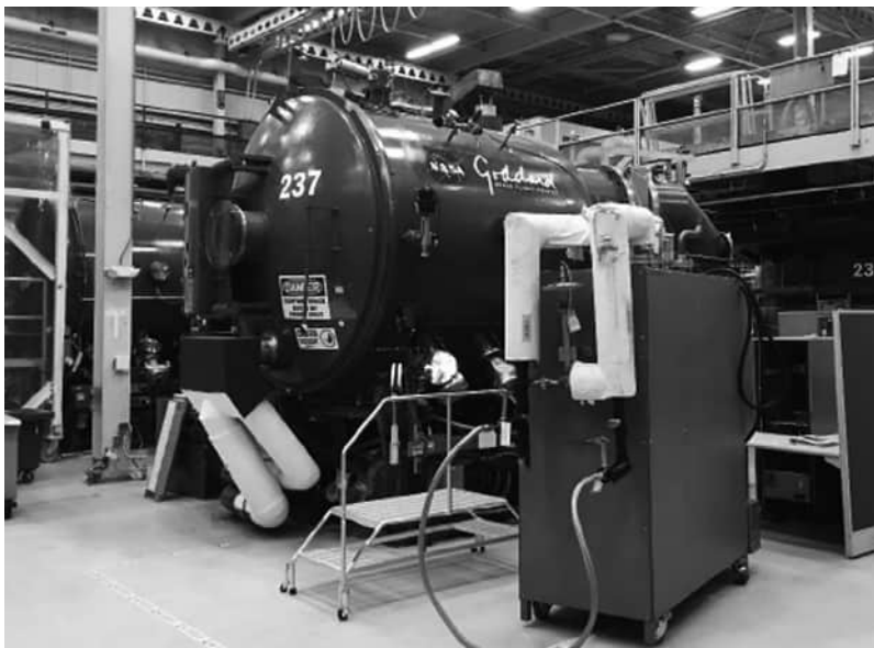
FIGURE 7.19 One of several thermal vacuum chambers at NASA Goddard Space Flight Center for testing of materials, systems, and components under different environments. Source: J. Fesmire
