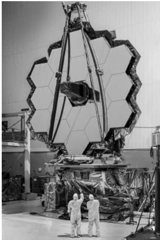
FIGURE 7.17 James Webb Space Telescope being prepared for vacuum chamber test. Source: NASA
