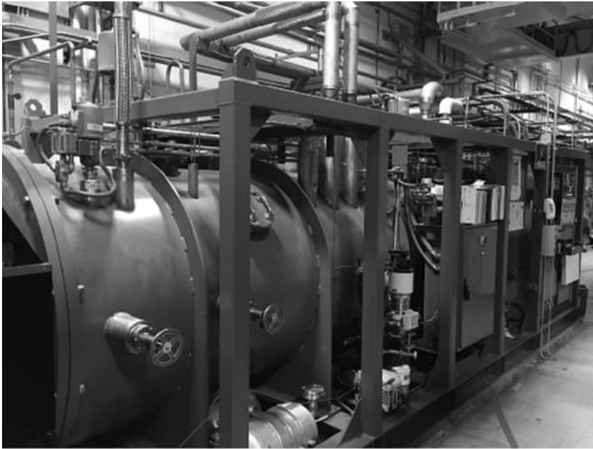
FIGURE 7.20 Cold box vacuum chamber for a hydrogen liquefier at NIST Center for Neutron Research in Gaithersburg, Maryland, USA. Source: J. Fesmire
