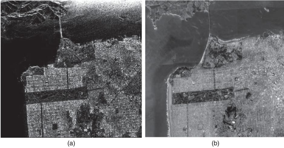
Figure 1.6 (a) NASA/JPL AIRSAR image for San Francisco Bay and the optical version, from Google Earth (b). The SAR image has spatial ground resolution of about 6.6 m in range and 9.3 m in azimuth. The images have not been registered (aligned) and some additional differences between them are due to geophysical corrections applied to the SAR data. Acquisition dates are not either the same. Source: (a) NASA/JPL AIRSAR and (b) Google Earth.
