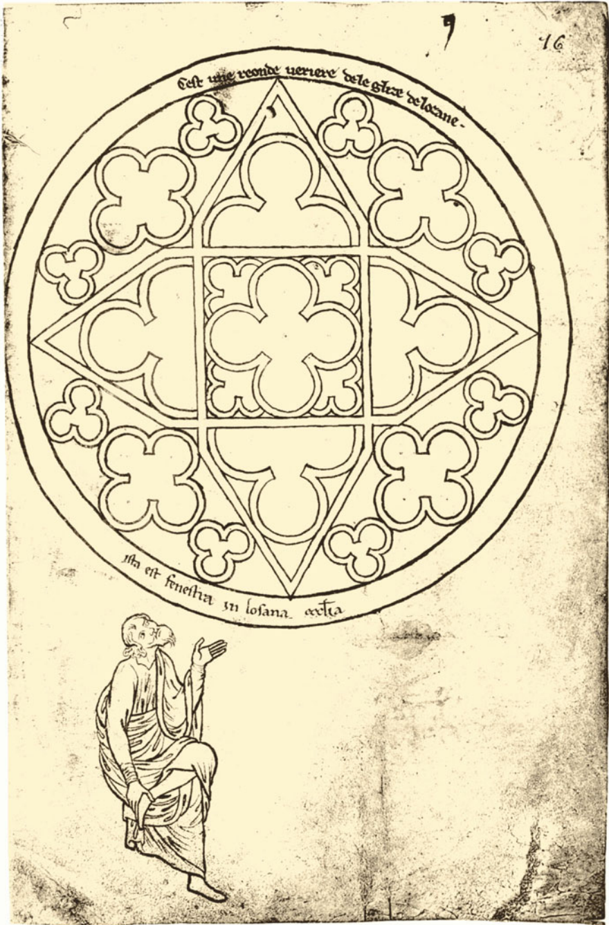
Illus. 4.4.1 From Villard d' Honnecourt's sketchbook (1230-35): Church window of the Early Gothic Cathedral of Lausanne (consecrated in 1275) [Villard d' Honnecourt Album. Paris, nd]
