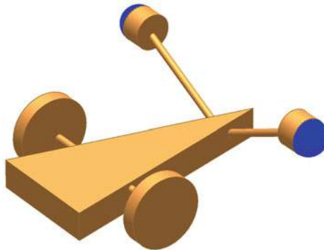
Fig. 2.12 A schematic diagram of the type of vehicle that Braitenberg [1] introduced. The vehicle consists of a pair of light sensors and a pair of wheels each of which is driven by its own motor
