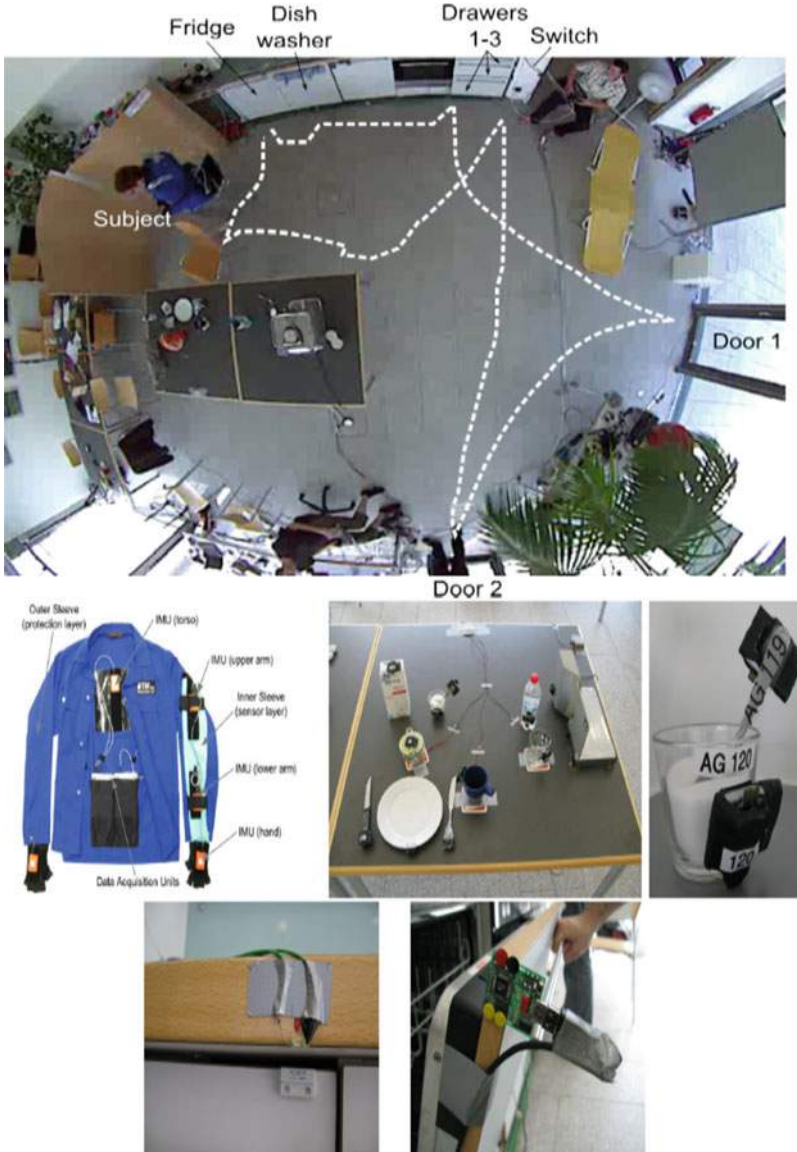
Fig. 3 Setup, wearable, object, and ambient sensors
