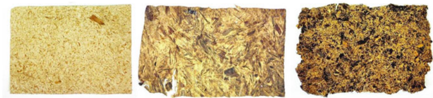
Fig. 4 Handmade paper made by artisans of various waste (Pineapple crown, banana trunk and coffee pulp) (photographs taken in Veracruz, Mexico)
