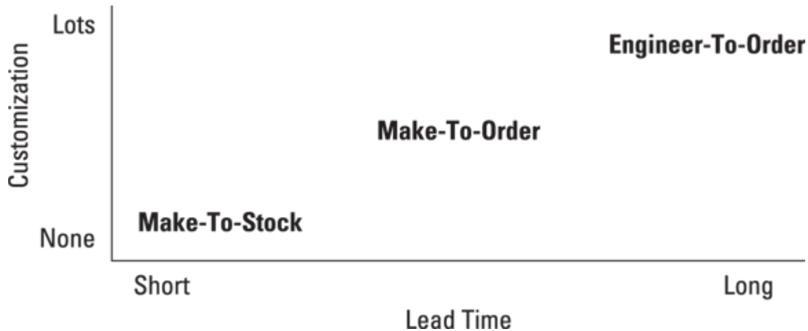
FIGURE 7-4: Make-to-stock, make-to-order, and engineer-to-order production.
