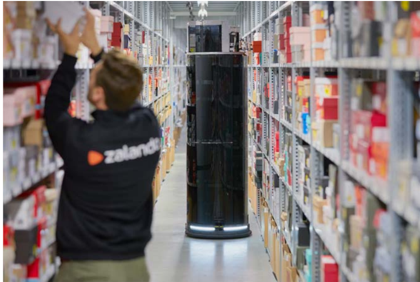
FIGURE 3.3 Collaborative order-picking employing Toru and human operators. Credit: Magazino GmbH, Oliver Jung.
