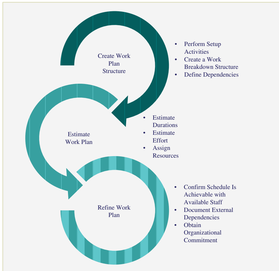
Figure 15–22. Activities required to develop a work plan. Source: © Deloitte & Touche LLP and affiliated entities.
