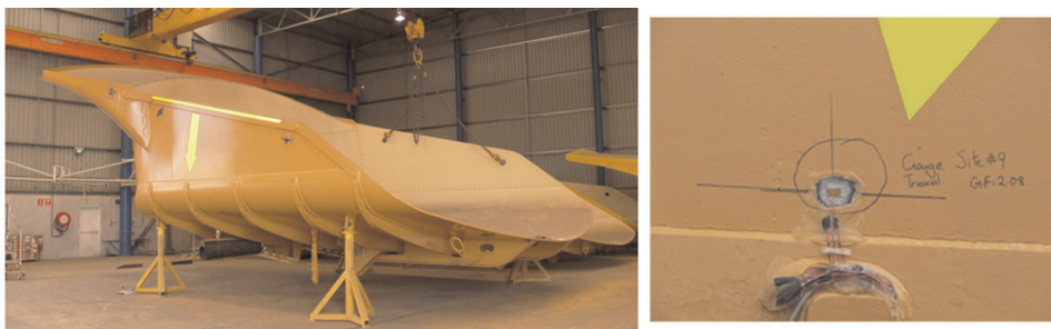
Figure 6. Mining truck tray and its critical location identified from strain gauging.
