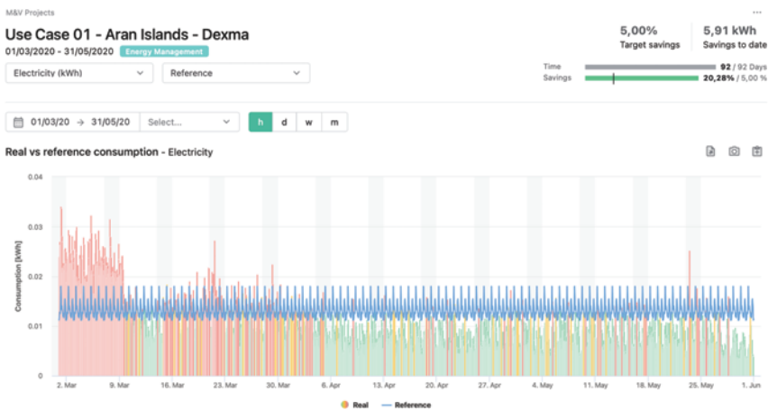
Figure 16.4 Example of M&V output from DEXMA platform (blue line – baseline, green bar – lower than baseline consumption, orange bar – close to baseline consumption, red bar – higher than baseline consumption)
