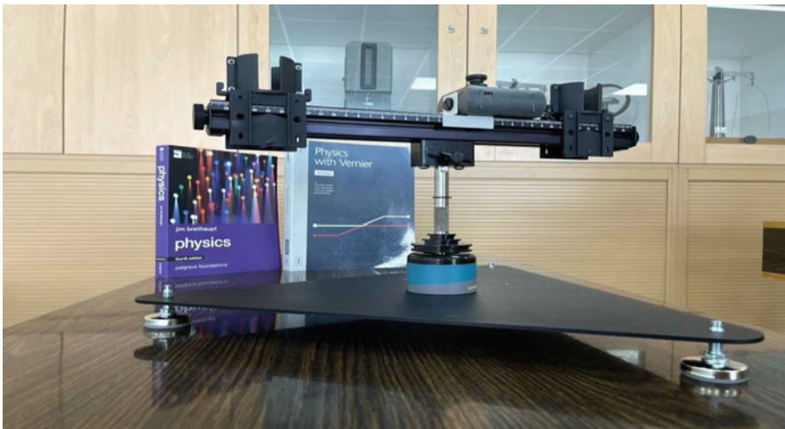
Fig. 2 Image of measuring GDX system for centripetal force [5]
