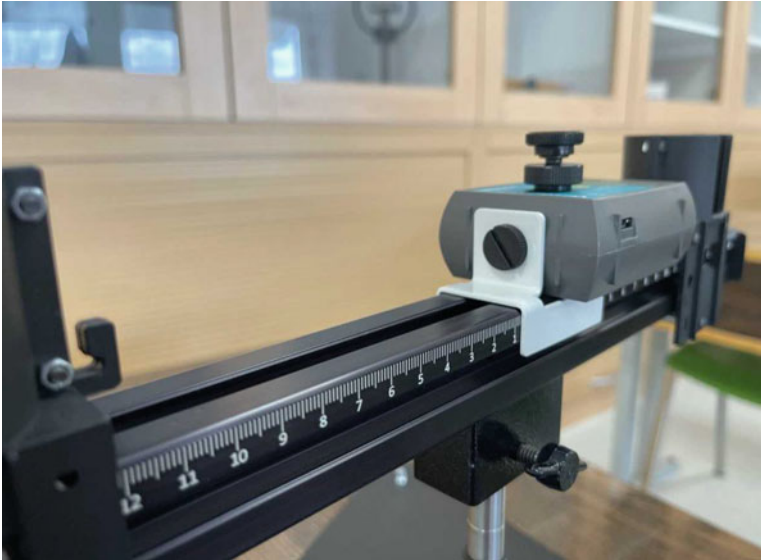
Fig. 3 Movable trolley on GDX system frame [5]
