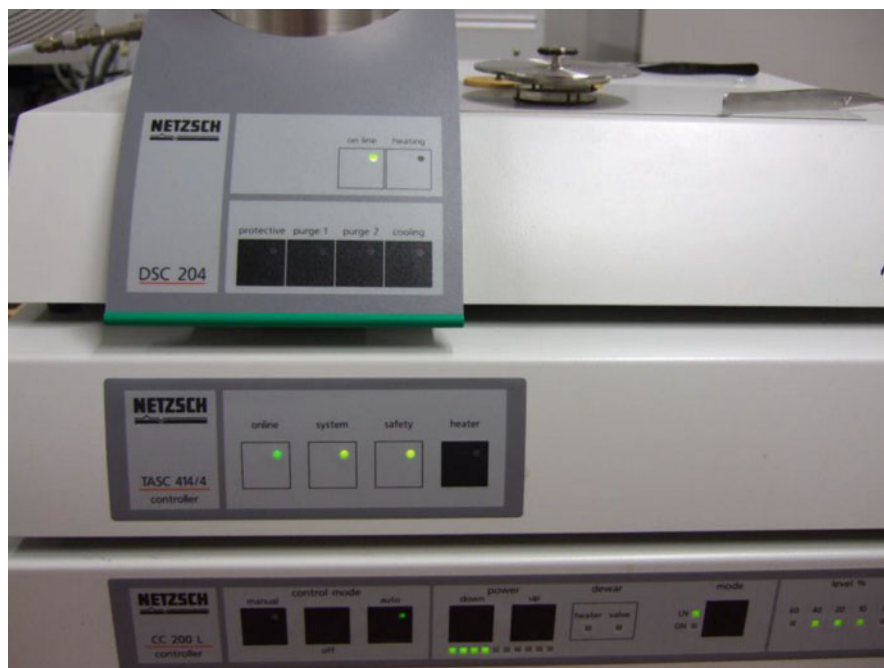
Fig. 4 Differential scanning calorimetry equipment NETZSCH. [Authors' own processing]
