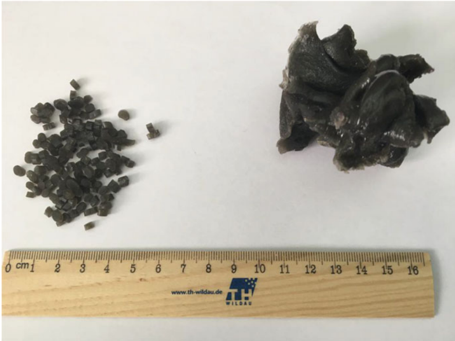
Fig. 3 Recycled polyvinyl butyral (left—granulate, right—homogenized material). [Authors’ own processing]
