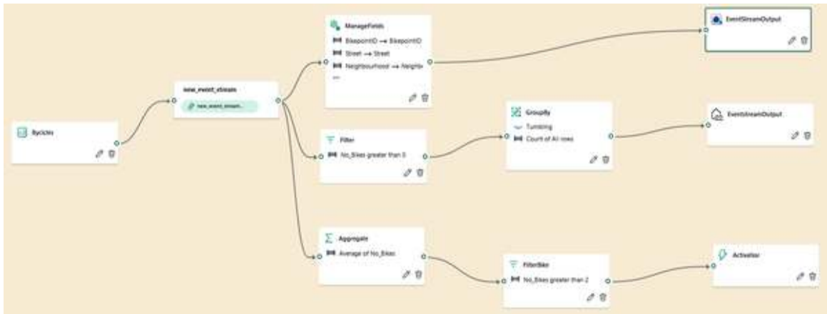
Figure 8-5. Common workflow for ingesting data with eventstream
