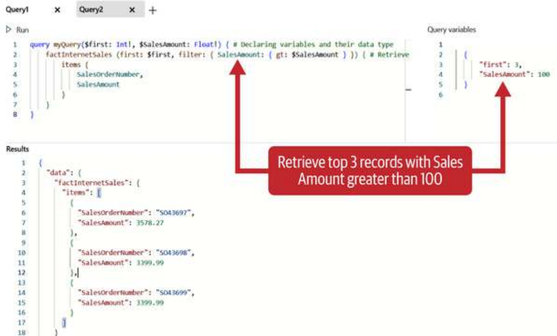
Figure 12-9. Passing multiple values dynamically to the query operation
