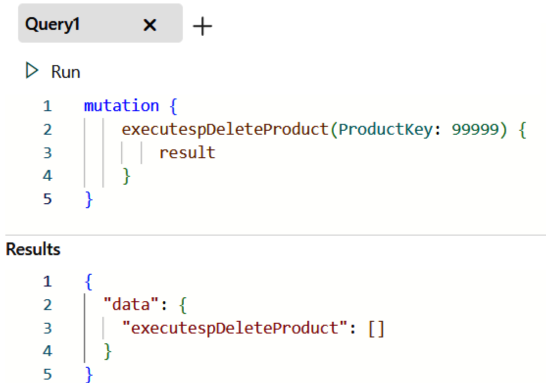
Figure 12-6. Deleting a record from the table by executing the stored procedure
