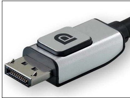
FIGURE 1-15: DisplayPort is a modern alternative to HDMI.
