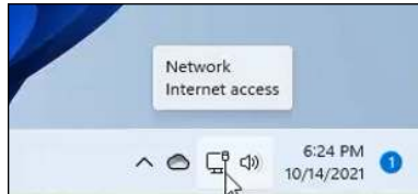
FIGURE 5-2: Your desktop PC is connected to the network and the internet.
