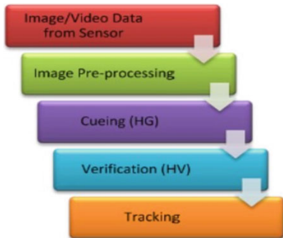
Fig. 4 Vehicle identification and monitoring system stages
