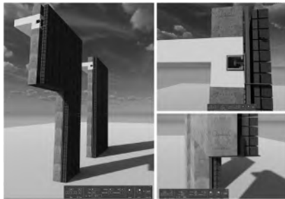
(b) The Masonry Brick Veneer cladding in VR.
