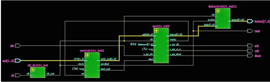
Fig. 11 FPGA architecture of the implemented tilt module: an SPI protocol was used to collect the data. The control block generates the clock and the address signals needed for computation [40]
