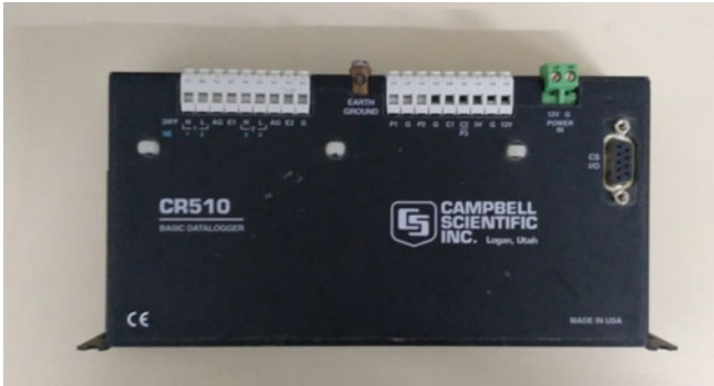
Fig. 15 Example of a commercial datalogger. The CR510 programmable datalogger is a basic solution from Campbell Scientific that has one digital input and four analog inputs, and it is programmed via the PC200W programming software
