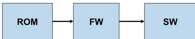
Figure 5-2. Simple block diagram showing the flow of booting up in a typical computing system
