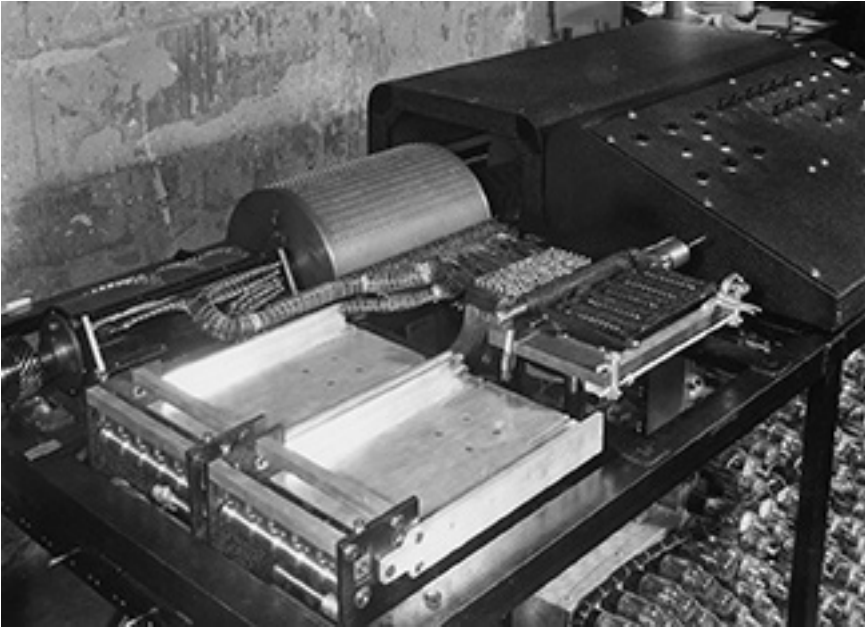
Last known photograph of the ABC computer before being dismantled by officials at Iowa State. (Image Courtesy of the Charles Babbage Institute Archives, University of Minnesota Libraries, Minneapolis)
