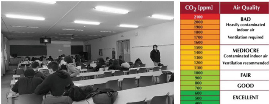
Fig. 6 Display of data on the screen and legend and instructions poster of the actions to be taken with the ventilation according to the measured CO 2 concentration
