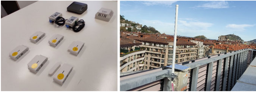
Fig. 7 Deployed open- source IoT monitoring system in the Campus of Gipuzkoa of the University of the Basque Country (UPV/EHU). Left, monitoring nodes and server. Right, deployed IoT LoRaWAN gateway
