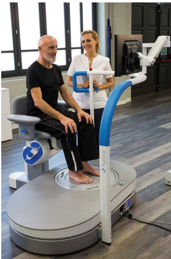
Fig. 3 Features of the hunova robotic platform include valuable solutions for neuromotor rehabilitation (especially effective for elderly) with diagnostic-prognostic functions too (e.g., predicting the risk of fall). Photograph: a patient on hunova. Courtesy of Movendo Technology. www.movendo.technology
