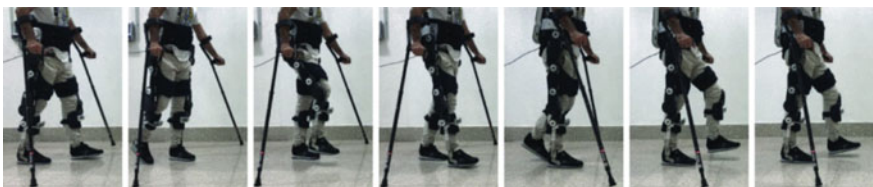
Fig. 6 Testing of the TWIN exoskeleton. Image adapted from [50]
