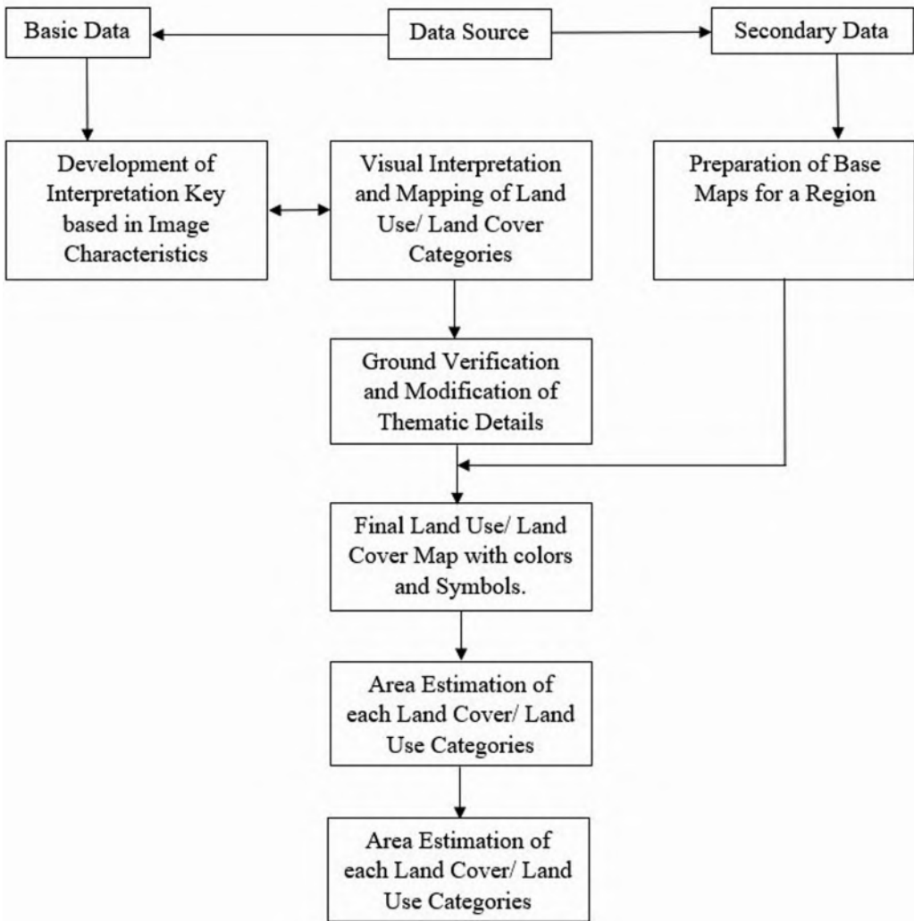
FIGURE 9.9 IoT remotely sensed image interpretation process for land use/land cover.
