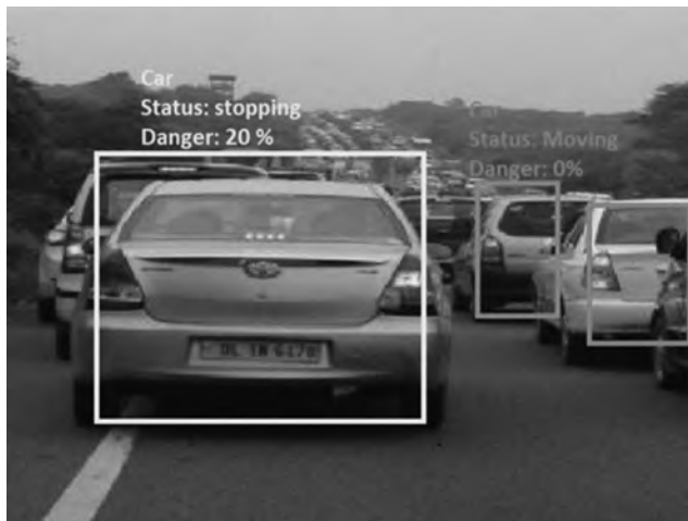
FIGURE 8.12 Algorithm determining the status of surrounding vehicles.
