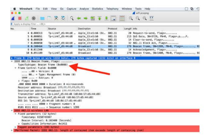
A beacon packet is a periodical packet that is sent by the access point (AP) on the network to provide information and to notify the AP presence in the network. In the filter toolbar, enter  $wlan.fc.type\_subtype == 0x08$ . The beacon packet cycle (in this case, equal to the default value, 100 ms) is displayed, as shown in the figure below.
