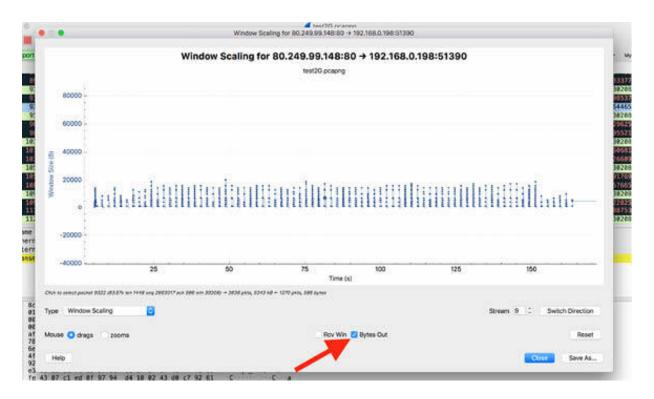
In general, as data is taken out of the receive buffer, the receive window should increase. From the previous figures, you can see that the receive window does not increase. Eventually, the transferred data fills up the receive window, and the data transfer stops until the receive window opens up again.
