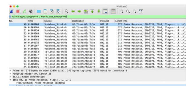
To display only a specific channel, in the filter toolbar, enter radiotap.channel.freq==2452. This display filter is based on the radiotap header. The channel frequency information is displayed in the Packet Details pane, as shown in the figure below.
