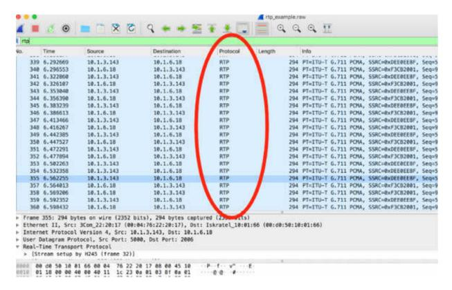
RTP provides end-to-end transport functions for real-time data such as audio, video, or simulation data over multicast or unicast network services. Realtime Transport Protocol (RTP) is defined in RFC 3550.
