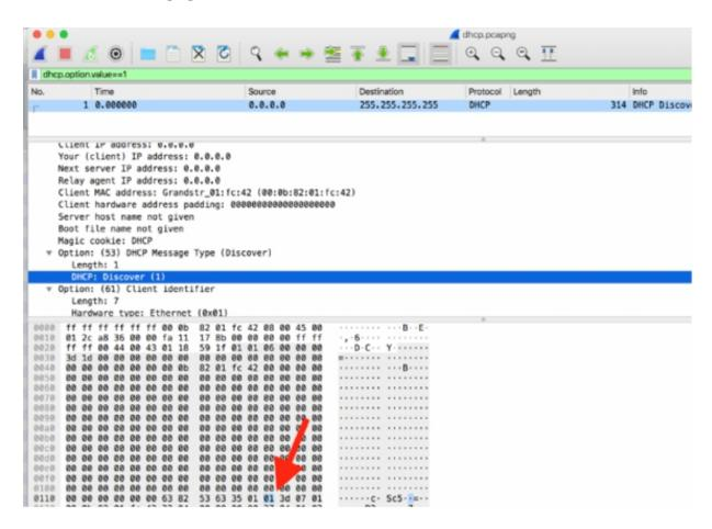
To display all DHCP offer packets in the Packet List pane, in the filter toolbar, enter dhcp.option.value=2.
