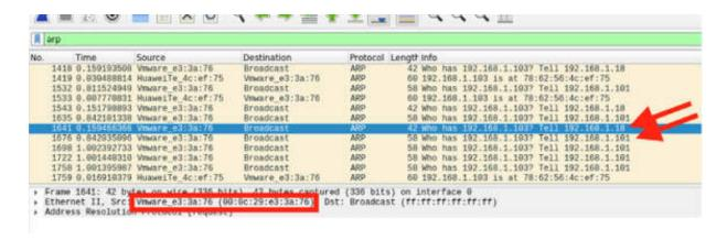
In this case, a host updates its ARP tables based on the information learned during the ARP poisoning process. When it wants to send data to another IP address, it consults its ARP table and forwards the packets to the MAC address associated with the target IP address.
