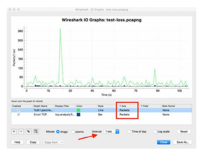
In the standard graph mode, you can add more than one traffic channel by clicking the add (+) button, as shown in the figure below.
