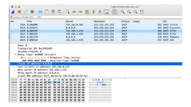
The "Your (client) IP address" field is the next field. It indicates the address offered by the DHCP server. Only the DHCP server fills in this field.
