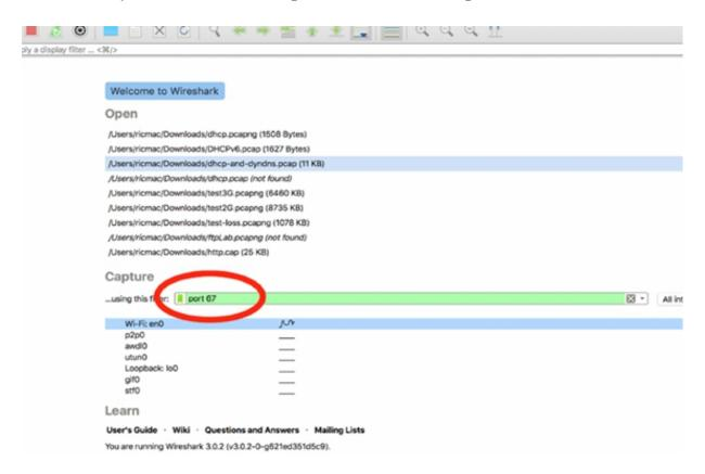
To display only DHCP packets in the Packet List pane, in the filter toolbar, enter dhep.
