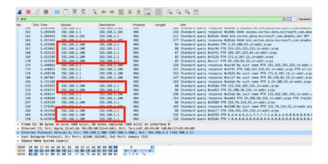
You can see that the host running Wireshark is capturing traffic on an Ethernet network and sending DNS PTR queries for each captured IP address. Besides making Wireshark visible, this traffic may overwhelm the DNS server if the capture contains a high number of IP addresses.
