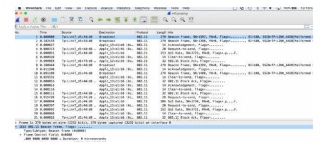
In the Packet List pane, select packet #5. In the Packet Details pane, open the tree view to see the packet details. As shown in the figure below, you can verify that this is a data frame. Data frames are the only WLAN frame types that can be forwarded to the wired network.
