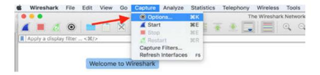
The Capture Options dialog box is displayed, showing all network interfaces available. The Wi-Fi network card is displayed with the header Ethernet, as shown in the figure below.
