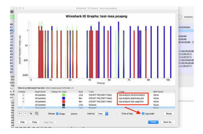
This advanced I/O graph illustrates the relationship between lost packets, duplicate ACKs, and retransmissions.
