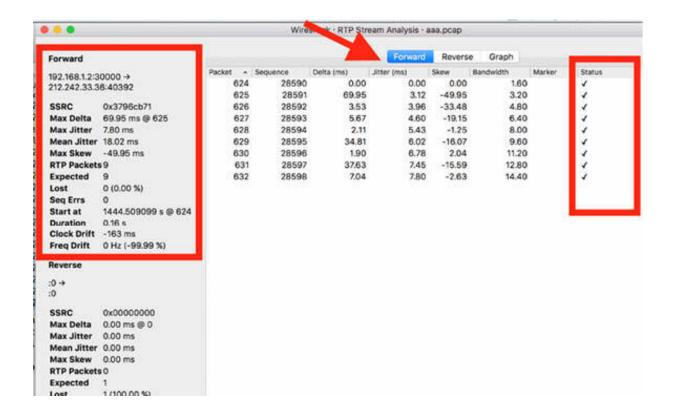
Packet loss can occur because of timing issues such as excessive jitter or clock skew between the VoIP endpoints. The Delta (ms) column in the figure above shows the time since the last RTP packet was received. This time should remain fairly consistent, but this is not the case (you can note a max of 69 ms and a min of 1.90 ms).
