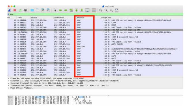
The structure of a POP packet is very simple. POP requests consist of a request command and a request parameter. POP responses consist of a response indicator and a response description.
