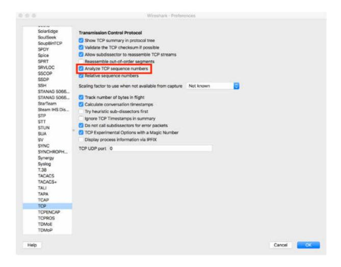
If you disable the above feature, the Expert Information related to these TCP conditions is automatically disabled. This feature is used to identify particular TCP conditions such as:
