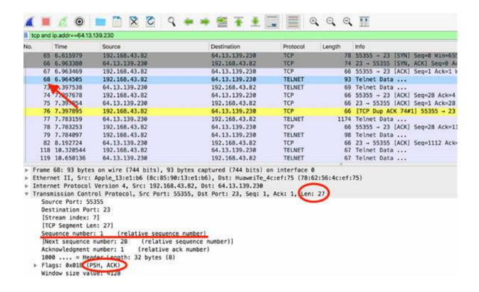
In the figure above, in the Packet List pane, packet #68 is selected. It has a length of 27 bytes and sequence number 1. Applying the sequence numbering equation, the sequence number should be 27 + 1 = 28. In the figure below, details of packet #73 are displayed with the highlighted data of interest.
