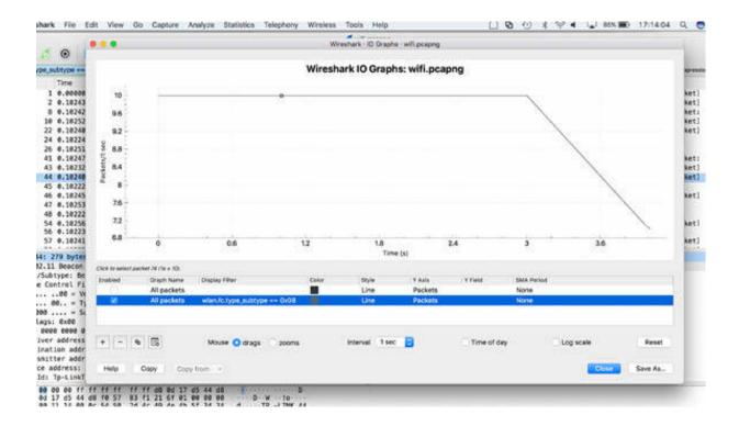
This graph shows that the period of beacon detection is quite constant until 3 seconds of capture after which either the capture is too short, or there is a problem where the access point stopped beaconing for a period.
