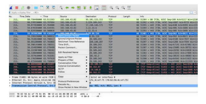
As a result, you can see all marked packets in the Packet List pane. You can also return to any of these packets at a later stage by using the Next Mark or Previous Mark options from the Edit menu.
