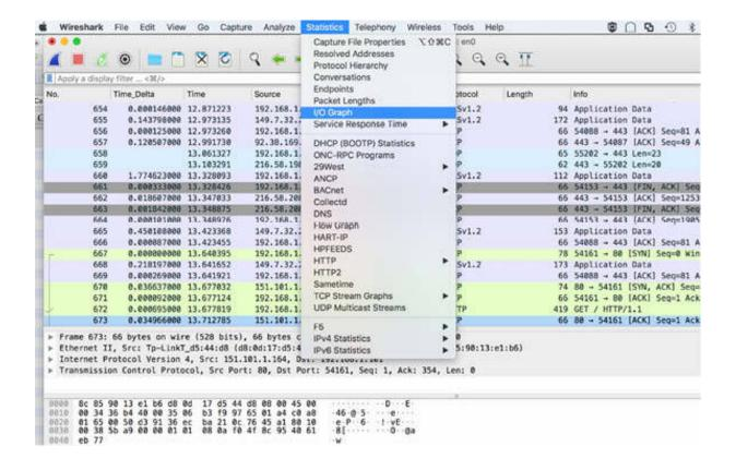
In the generated I/O graph, apply a TCP filter to identify only a single transmitter (ip.src == x.x.x.x). To depict the traffic payload, in the "Y Axis" field, select AVG(\*) Y Field, and in "Y Field", enter tcp.len, as shown in the figure below.
