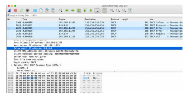
The "Client MAC address" field is the next field. It contains the MAC address of the client. This is a useful field to filter on if a user complains about the boot-up process, and you suspect it might be a DHCP problem.
