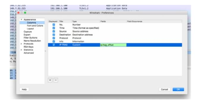
If the fragmentation offset value does not increment with each new fragment, the entire communication is considered suspicious. For example, if the ip.frag\_offset column indicates that the fragment offset values are 0, 1480, 2960, 4400, 1480, 5920, 7400, and 8880, you must wonder about the fifth packet in the set. If it is not retransmission, perhaps you have the IP fragment override situation.
