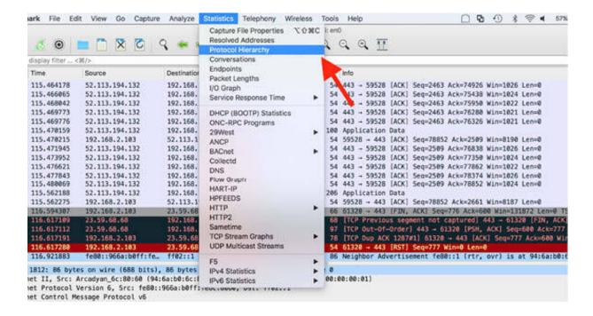
The Protocol Hierarchy Statistics dialog box is displayed. It shows the statistics in percentage and bytes for each protocol, as shown in the figure below.
