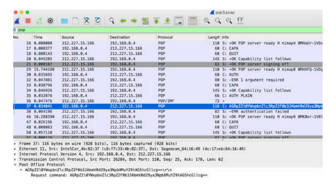
The password, however, is incorrect. As a result, the server issues the "Authentication failed" message (packet #38).
