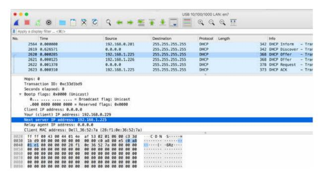
The "Relay Agent IP address" field is the next field. It shows the address of the DHCP relay agent (if one is in use).
