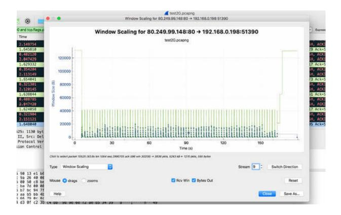
To clearly see the periodic window size, zoom in, and select the "Rcv Win" check box, as shown in the figure below.
