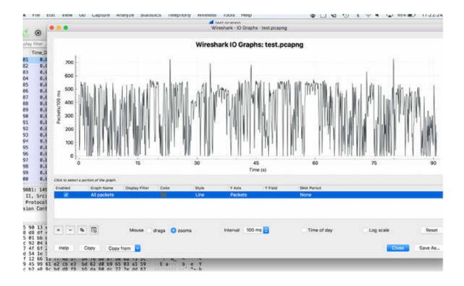
The heartbeat effect is indicated in the I/O graph. Various misconfigurations can affect network performance. For example, video multicast traffic—having a lower priority than the file transfer, voice, and email traffic—may be held in queues along a path while the higher priority traffic flows ahead of it.
