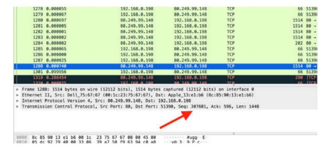
The TCP Time Sequence graph's data moves in one direction. Therefore, in the Packet List pane, make sure that you select a packet that contains data or that is traveling in the direction of data flow.
