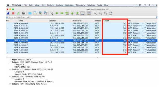
In the Packet List pane, observe that the DHCP packets have variable lengths, as shown in the figure above.
