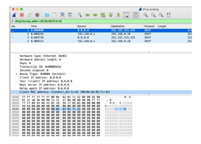
To identify a DHCP ACK message to the client using IP address 192.168.0.10, in the filter toolbar, enter (dhcp.ip.your==192.168.0.10) && (dhcp.option.value==05).
