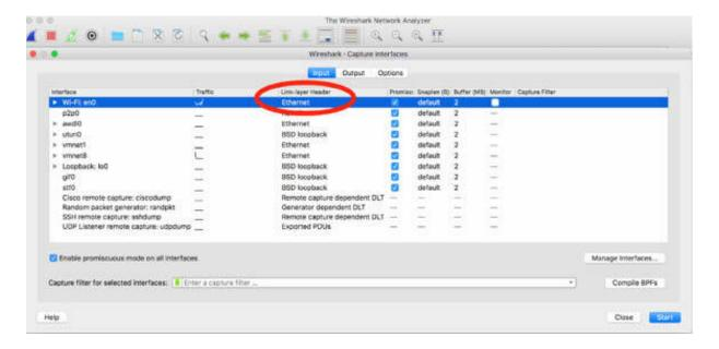
In the Wi-Fi network card row, select the check box in the Monitor column, as shown in the figure below, and click Start to begin the network capture.
