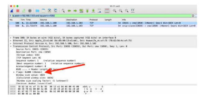
To detect null scans, you can create a coloring rule or a display filter (tcp.flags==0x000) for TCP packets for which no TCP flags are set.
