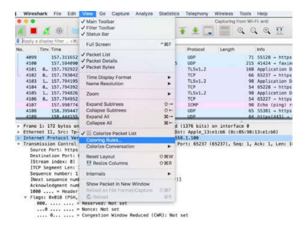
The Coloring Rules dialog box is displayed. You can add a new filter to clearly display the unusual packets in the Packet List pane. For example, to highlight the unusual ICMP Echo Request used by NetScanTools, create a coloring rule by using the syntax (icmp.type==8) && !(icmp.code==0x00), as shown in the figure below.
