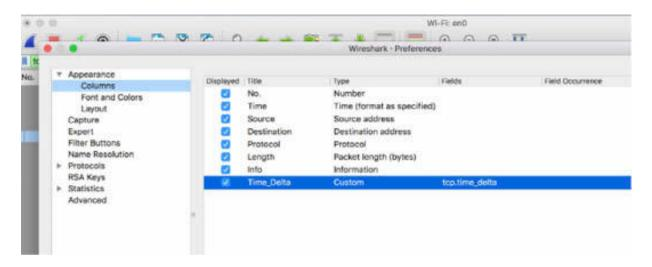
To view the roundtrip latency times of the TCP connections, sort the Time\_Delta column by clicking the column header. The results, shown in the figure below, indicate that a few connections have a very high round trip latency (over 700 ms, packets #4075 and #4078).
