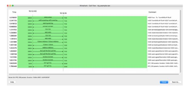
On the left side, the timeline is displayed which is followed by the source and destination addresses. Each message of the flow is displayed by using an arrow. Selecting a message and clicking on it displays the related packet in the Packet List pane, as shown in the figure below.
