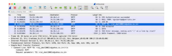
The DATA command (packet #20) indicates that the client is ready to send the email, and if the server is ready (as in this case), it responds with 354 Start Mail Input. Now the client can send the email to the SMTP server. In this case, the message is split into three segments, as shown in the figure below.
