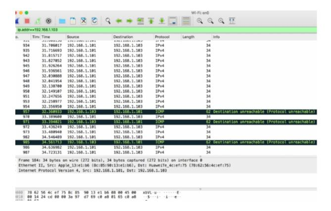
To detect IP protocol scans, you can create a coloring rule or a display filter (icmp.type==3 && icmp.code==2) for ICMP Type 3/Code 2 packets. This will allow you to detect a lot of ICMP packets in the capture.
