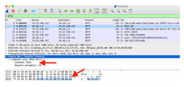
In the Packet List pane, select packet #22. In the Packet Details pane, open the tree view to see the details. The DATA message, highlighted in the figure below, initiates the email data transfer.
