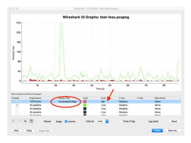
You can set different colors for the channels used for graphs. In general, it is useful to stick to the standard color codes: green for good; red for bad.
