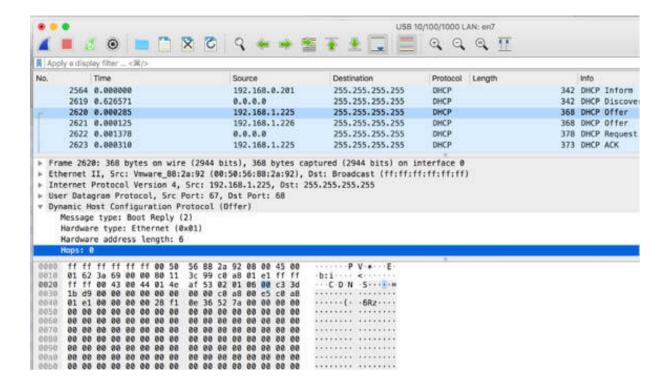
The "Transaction ID" field is the next field. It is used to match the DHCP request and response packets.
