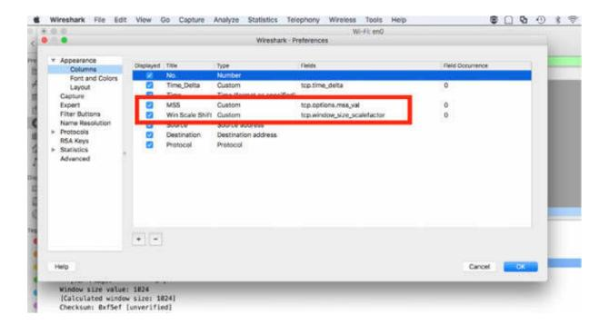
Apply a TCP or ICMP filter, as shown in the figure below, and then sort the results based on the MSS column.
