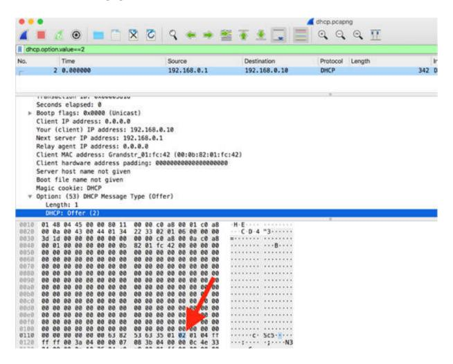
To display the DHCP messages that contain the MAC address 00:0b:82:01:fc:42, in the filter toolbar, enter dhcp.hw.mac addr==00:0b:82:01:fc:42.
