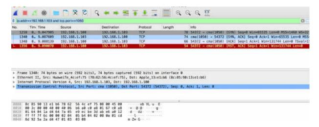
Based on the Packet List pane shown above, it is clear that the scanner completed the three-way handshake. The scanner sends the ACK packet in packet #1348. This is a classical pattern of a TCP full-connect scan.
