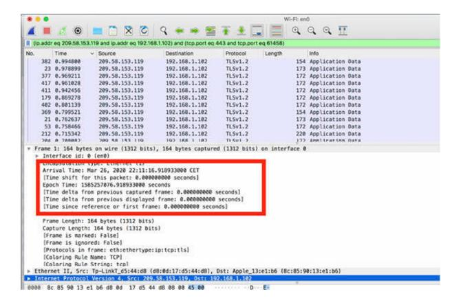
You can see numerous time values inside the Frame field. Although these values are not the actual fields in the packet, Wireshark can find packets based on these values.
