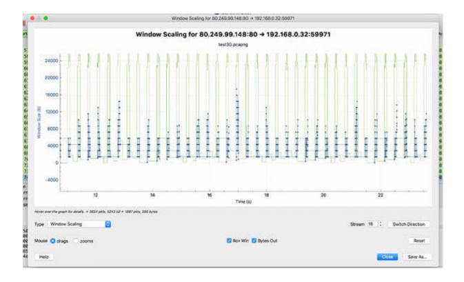
Zoom into the graph shown in the figure above to analyze it and compare it with the graphs from the earlier tasks. You will observe that the TCP window has not been saturated by the data flow, and there are no TCP Window Full messages in the Packet List pane.
