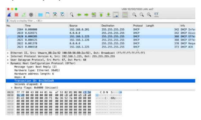
The "Seconds elapsed" field is the next field. It indicates the number of seconds that have elapsed since the client began requesting a new address or renewal of an address. You may notice an error warning from Wireshark when a vendor sets this field using the little-endian format. Wireshark interprets the field based on the big-endian format but provides a note indicating the difference.
