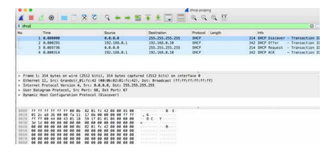
To display all DHCP discover packets in the Packet List pane, in the filter toolbar, enter dhcp.option.value==1.
