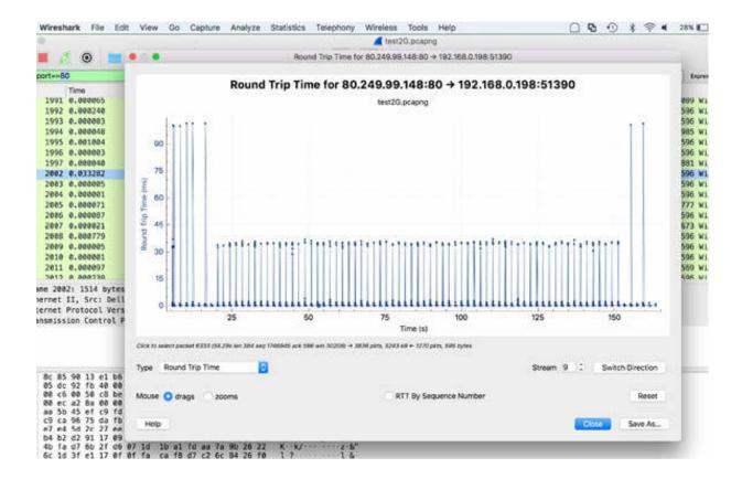
Considering that the trace file is related to a data transfer and the Y axis defines the round trip time in milliseconds and the X axis defines the time in seconds, you can observe that the latency time is quite constant and does not present high values.
