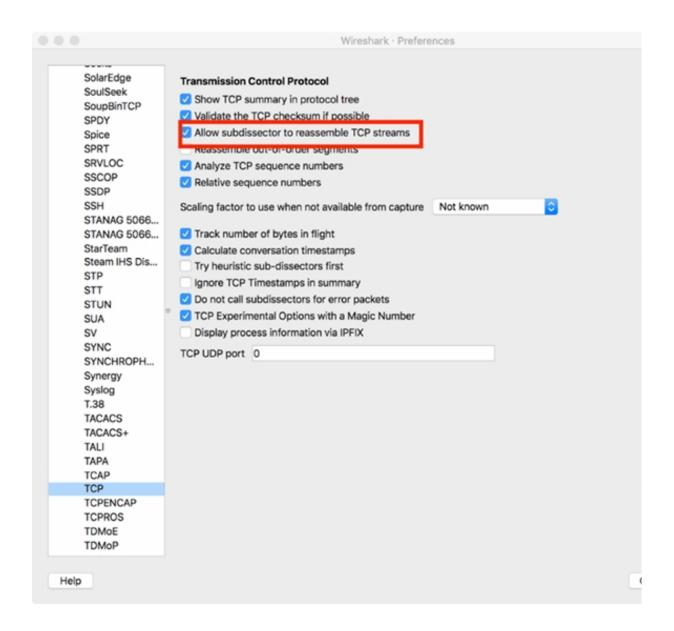
When working with a TCP data stream, you can choose to have Wireshark reassemble the stream and provide links to each packet containing data from the stream. When enabled, this setting also alters the display in the Packet List pane.
