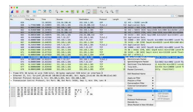
The Follow TCP Stream dialog box is displayed in which the server indicates to the client that it must connect to "nytimes.com". This prompts the client to generate a DNS query for the new website before generating a TCP handshake.
