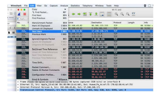
Examine each packet with the large TCP delta time, and apply a TCP conversation filter to see what's happening, as shown in the figure below.
