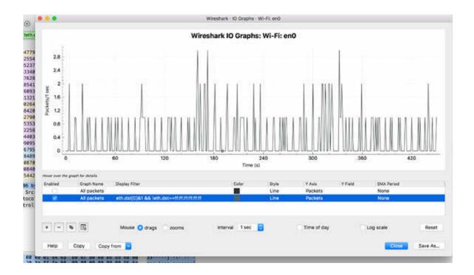
When baselining such types of traffic, you need to identify who is transmitting broadcast/multicast traffic and from which applications. The I/O graph provides the typical rate in packets per second. This is required for identifying an increase or decrease in the traffic in a future captures.
