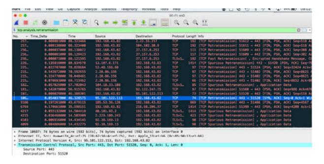
In the figure above, you can see a lot of TCP retransmission packets, indicating that the performance of the communication is getting low.
