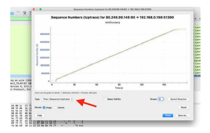
TCP headers contain a "Sequence number" field (as you experimented in previous labs) that increments by the number of bytes sent during data transfer. If a TCP header sequence number is 1000 and there are 200 bytes of data in the packet, the TCP header from this source should contain the sequence number 1200. If the next packet again contains the sequence number 1000, this is a retransmission packet. If the next TCP packet contains the sequence number 1400, a segment must have been lost.
