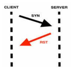
If a lot of failed TCP connections are present in a network capture, it could be an indication of a TCP scan in progress.
