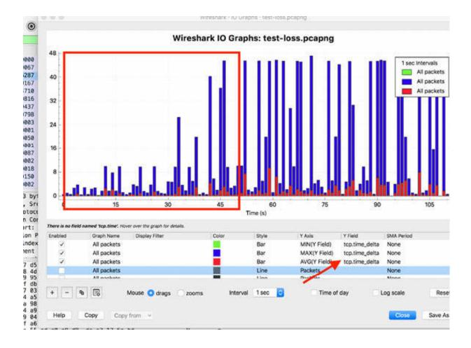
As shown in the figure above, there is a time region where an increase in the round-trip latency time is visible.
