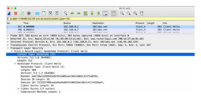
The TLS handshake enables peers to agree on security parameters for the exchange of data and to authenticate themselves. In addition, errors during the handshake process are relayed in the TLS handshake packets. The handshake process usually includes the following:
