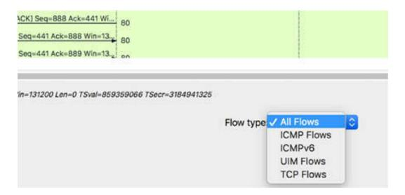
The general flow view includes application-layer information, such as requests and replies. The TCP Flow graph shows the TCP header values, such as the sequence number and acknowledgment number values and the TCP flag settings.
