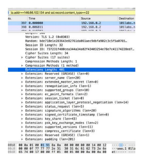
The server name extension provides the server name, which, in this case, is <a href="https://www.101labs.net">www.101labs.net</a>. The server name extension enables the client to create a secure connection to a virtual server that may be hosted on a machine that supports numerous servers at a single IP address.
