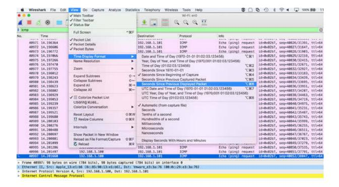
You can observe that the majority of the ping/flood packets are sent after 200 microseconds (millionths of a second) gap, as shown in the figure below.
