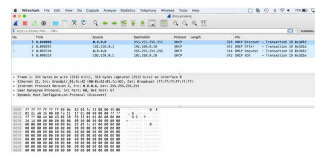
On the main menu, select Statistics > DHCP (BOOTP) Statistics to display the Statistics dialog box that summarizes the DHCPv4 message types in the trace file (currently, this feature does not support DHCPv6).
