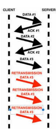
In the figure above, a situation during the normal data exchange is shown. For each exchanged data packet, the side receiving the DATA sends an ACK message to notify the reception. At a certain point, no ACK message is sent, and the sender retransmits the DATA (packet retransmission).
