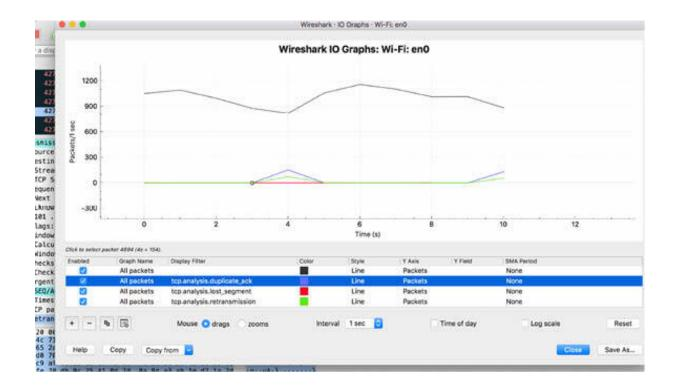
As shown in the graph above, there is no clear impact of packets lost during this quite short TCP session. In general, TCP doesn't do well with a large number of packets lost in a single congestion window, so it is important to keep an eye on this important parameter.
