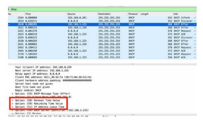
In the Packet Details pane, click each of these fields to open the tree view. The IP Address Lease Time (LT) defines for how long the client is allowed to use the assigned IP address. The Renewal Time Value (T1) is .50 LT, and the Rebinding Time Value (T2) is .875 LT.
