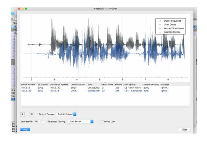
The RTP Player contains a playback graph for each stream detected. In the figure above, you can see two playback graphs—one for each direction of the call. Below the graphs, you can observe the information related to the source/destination address and port, the number of packets, the sample rate, and other useful information.
