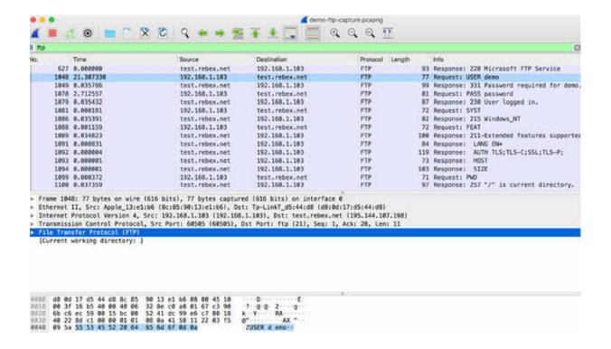
The FTP packet structure is very simple. The FTP commands follow immediately after the TCP header, as shown in the figure above. Some commands include an argument. The following list provides a list of commands that use arguments:
