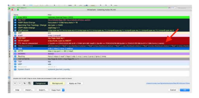
This coloring rule examines the destination IP address field to look for multicasts. Traffic is colored with a red background and a white foreground if it is not multicast but has an IP TTL value lower than 5 or if it is multicast and the IP TTL value is not equal to 1.
