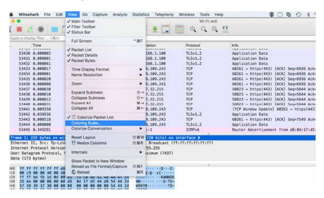
ICMP Redirect packets are also easy to spot during a live capture with a display filter (icmp.type==5).
