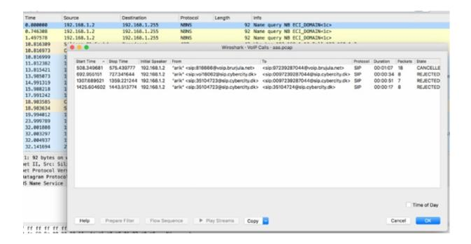
You can select a single call or multiple calls (by using the CTRL key). The "Play Streams" button is enabled after selecting a call.
