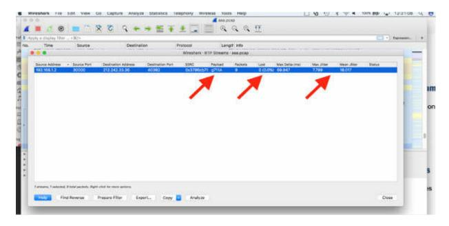
Select a communication flow, and click Analyze. Wireshark lists the packets in the RTP stream and provides additional details on the VoIP call. The Status column indicates problems in the RTP streams. The Forward tab is displayed in the figure below.
