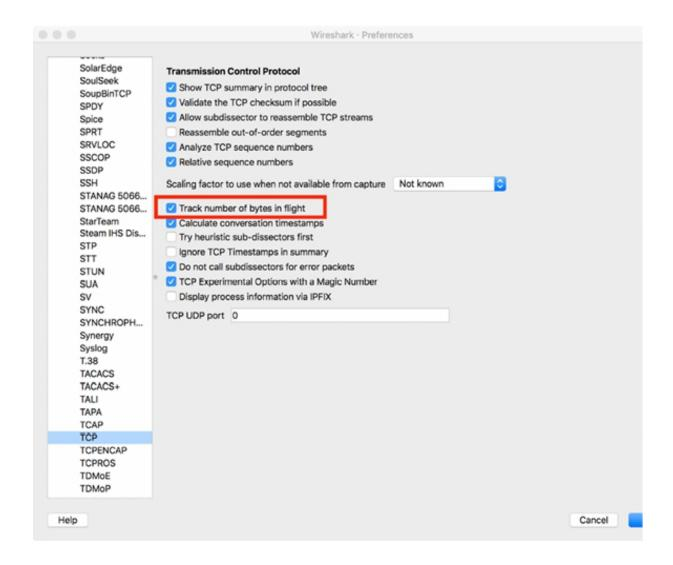
When this setting is enabled, you can create an I/O graph depicting the total number of bytes in the trace file and the number of bytes in flight by using the tcp.analysis.bytes\_in\_flight display filter value. This is particularly useful when you suspect that congestion window issues are slowing file transfer processes.
