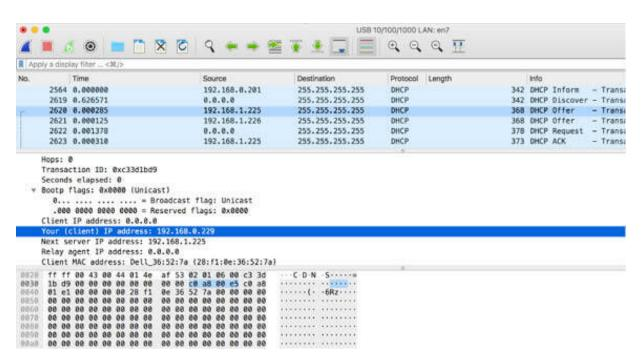
The "Next server IP address" field is the next field. It contains the address of the DHCP server when a relay agent is used.
