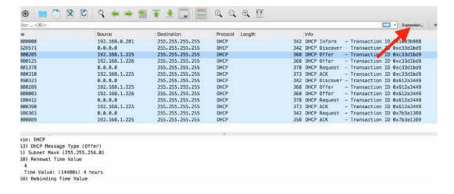
The Display Filter Expression dialog box is displayed. To view a list of all DHCP filters, scroll down and click the DHCP/BOOTP—Dynamic Host Configuration Protocol field to open the tree view. Manually create a more appropriate display filter.
