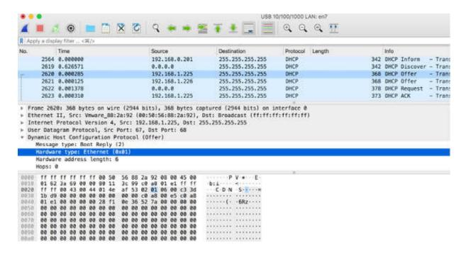
The "Hardware address length" field is the next field. It indicates the length of the hardware address, which is 6 for an Ethernet address.
