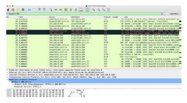
The filter for HTTP or HTTPS must be based on the port in use, such as port 443 for HTTPS (tcp.port=443). Alternatively, you can use the ssl display filter. HTTPS uses Transport Layer Security (TLS) which is based on SSL. If you use the ssl display filter, you will not see the TCP handshake process or ACK packets. Therefore, it is best to use a port number based display filter to see all packets in an SSL conversation.
