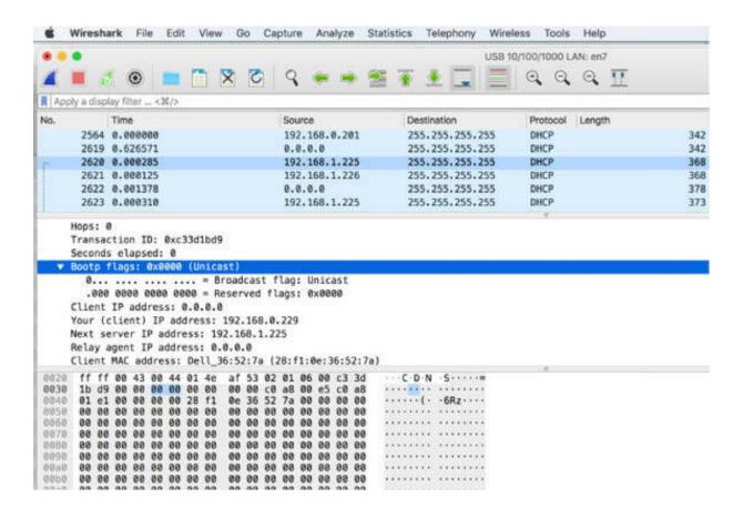
The "Client IP address" field is the next field. It is filled by the client when the DHCP server assigns an IP address to the client.
