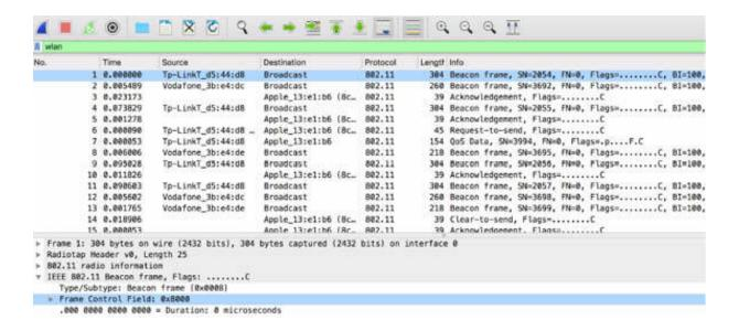
To display only beacon frames, in the filter toolbar, enter wlan.fc.type\_subtype==8, as shown in the figure below.
