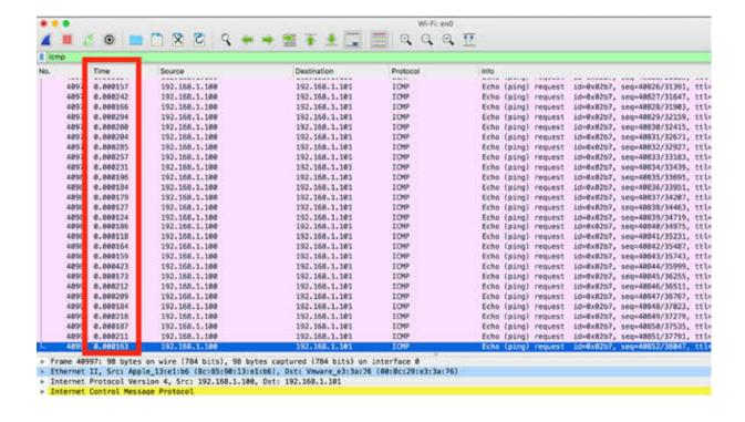
Such time values in the Time column are a clear indication of a flooding attack. If the flooding attacker is using Macof, it is important to know that it sends SYN packets to random target addresses. Macof has a signature in the TCP header of each SYN packet, so you can build the following coloring rule: tcp.window\_size==512 && tcp.flags.syn==1.
