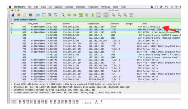
Remove the previous filter from the filter toolbar and select the packet immediately after the HTTP get request (packet #672). Right-click the selected packet and select Follow > TCP stream, as shown in the figure below.
