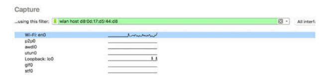
Capture the traffic for a few minutes. In the Packet List pane, only the filtered packets are displayed, as shown in the figure below.
