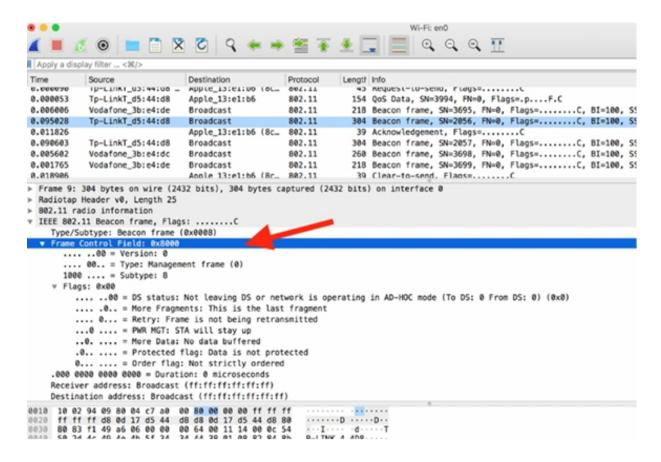
The Frame Control field is the first field of the 802.11 packet. It consists of 2 octets and contains numerous individual fields, as shown in the figure below.
