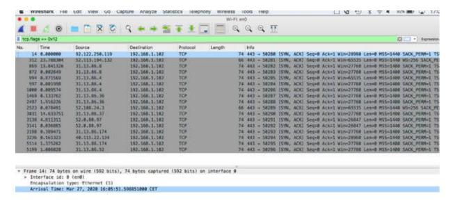
As shown in the figure above, only SYN/ACK packets are displayed.
