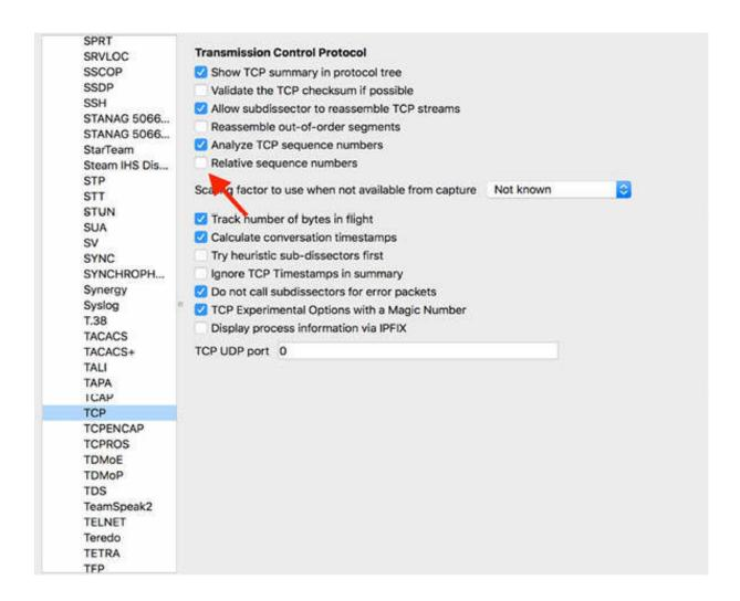
Wireshark displays the absolute sequence numbers that are, in general, big numbers. However, when analyzing a capture, it is easier to work with smaller numbers. The figure below shows the analysis of the same sequence numbers that you examined in the previous step but with the absolute value enabled.
