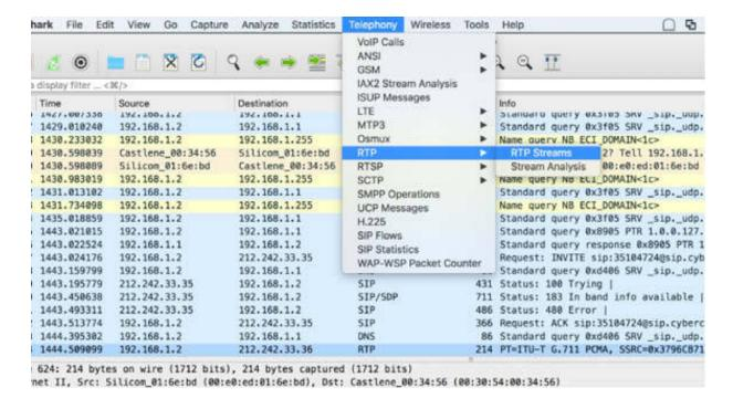
The RTP Streams dialog box is displayed, containing information related to packet loss, jitter, and payload for each communication flow, as shown in
