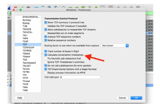
In the Preferences dialog box, add a column (Time\_Delta) for displaying the time since the previous frame in this TCP stream (tcp.time\_delta), as shown in the figure below.
