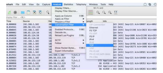
If you select a TCP conversation, the maximum gap is 0.99s, as shown in the figure below.
