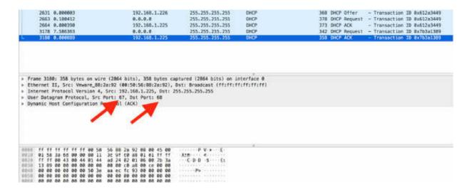
Depending upon the client's current configuration state and what the client wants to know from the server, the DHCP traffic can be different in terms of packets content. In the default startup of a DHCP client that is outside its address lease time, the Discover-Offer-Request-Acknowledgment sequence is used, as shown in the first sequence in the figure below.
