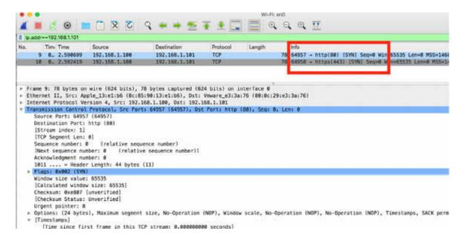
If a target blocks ICMP pings, you can use a TCP or UDP port scan to identify hosts on the network.
