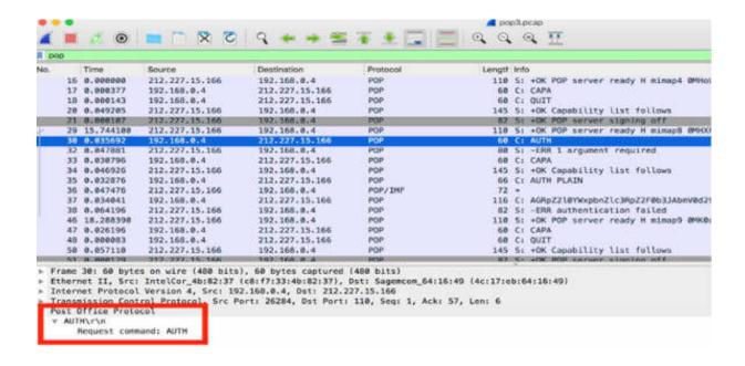
The client issues the AUTH Request command. As a response, the server sends packet #32, with response indicator "–ERR" and response description "1 argument required", as shown in the figure below.
