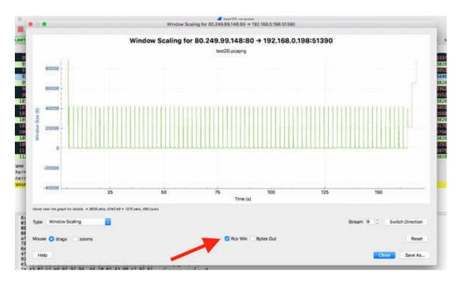
To identify the amount of data flowing with the TCP stream, select the "Bytes Out" check box, as shown in the figure below.
