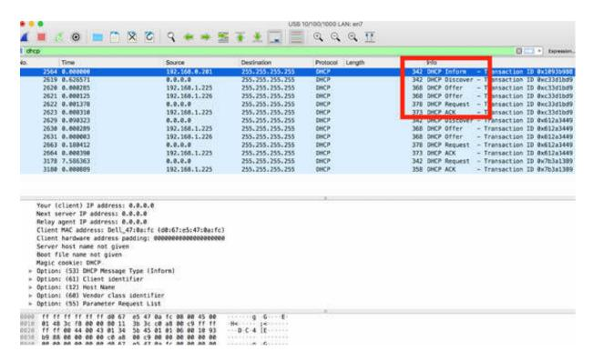
In the Packet List pane, select a DHCP Offer packet and inspect the Packet Details pane. As shown in the figure below, during the address request and assignment process, the client obtains the following three time values:
