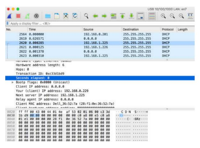
The "Bootp flags" field is the next field. These flags indicate whether clients accept unicast or broadcast MAC packets before the IP stack is completely configured. This field is not present in DHCPv6. The figure below shows the flags in the tree view.
