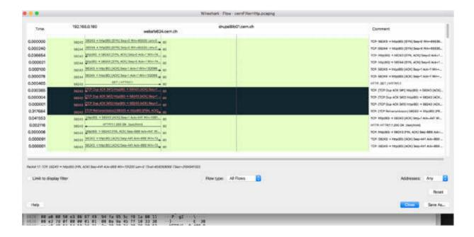
To customize the Flow graph, click "Flow Type" and select a type from the drop-down list, as shown in the figure below.
