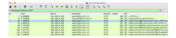
To display only a specific target host, in the filter toolbar, enter http.host=="info.cern.ch".
