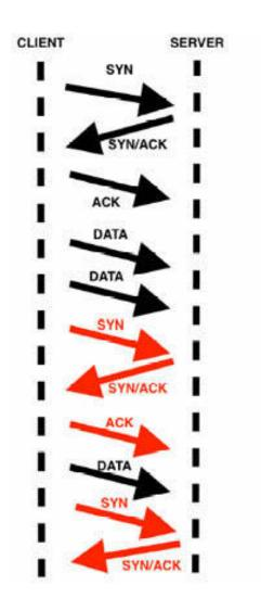
In the figure above, after a successful handshake process (SYN—SYN/ACK—ACK) and some DATA exchange between the client and the server, the handshake appears again. This could be because the connection is not stable in terms of physical stability.
