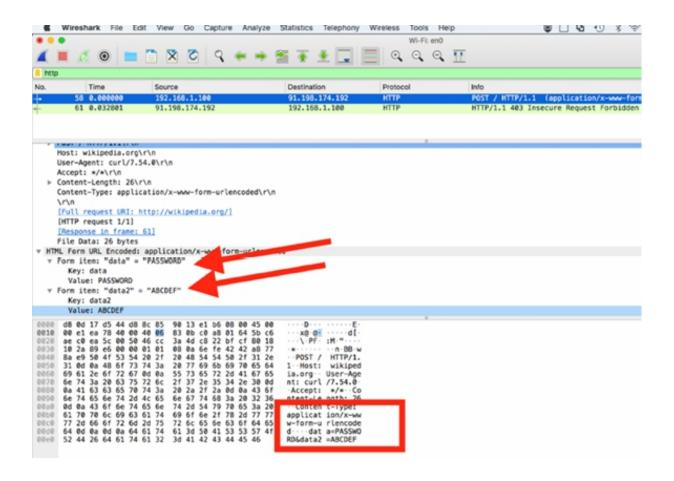
As shown in the figure above, you can easily spot the password "ABCDEF" in plain text. This confirms that one method to identify whether clear text passwords are crossing the network is to begin packet capture and then access the host using a password. You can also use the Find feature to look for a string in the trace file or follow the TCP Stream (or UDP Stream) to look for the password in a readable format.
