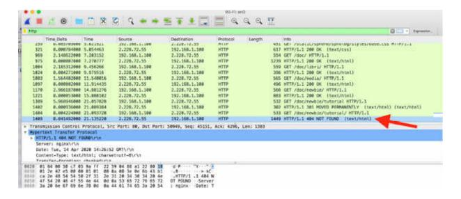
Open the I/O graph and in the "Display Filter" field, enter the source IP address of the website visited (in this case, 2.228.72.55) and verify that at a certain point, the server throughput has drooped to zero because the page doesn't exist. The result is displayed in the figure below. If you click on the point where the throughput is dropped to zero, you can jump to the related packet in the trace file.
