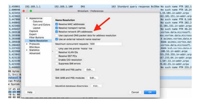
Capture the traffic on an active network interface for a few minutes. Stop the capture and save the file. In the filter toolbar, enter dns. You will observe a large number of DNS requests transmitted from the machine where Wireshark is running (i.e., ip src 192.168.1.100), as shown in the figure below.
