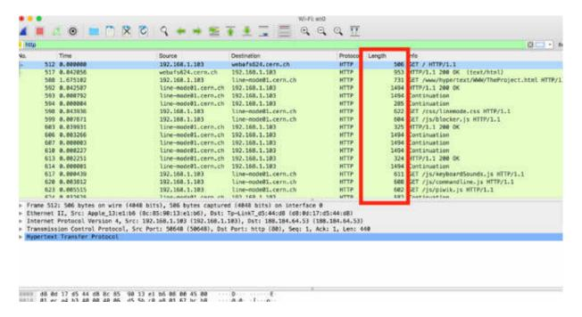
The results in the Packet List pane indicate that HTTP packets are of variable length. The HTTP request consists of a method that defines the purpose of the HTTP request. The HTTP response contains a numerical response code, referred to as a status code.
