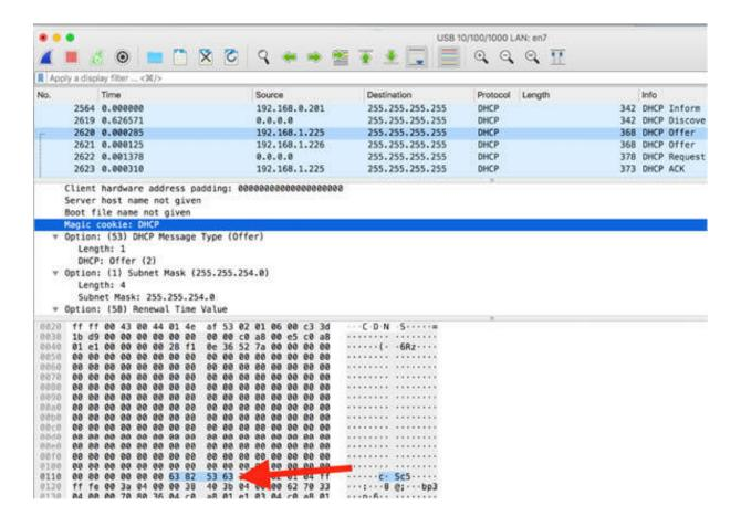
The Option fields are the last fields. The options are used to provide the IP address and configuration requests to the DHCP server and replies to the client. The following list contains some of the common option types:
