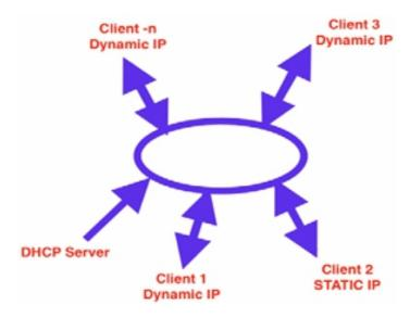
In this scenario, one or more hosts on the network have statically-assigned addresses and the DHCP server is unaware of this. In such a situation, the DHCP server may offer an address that is already in use in the network. This can cause a problem because two hosts with the same IP cannot exist on the same network. The figure below shows this problematic situation.
