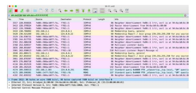
As shown in the figure above, there is a lot of multicast traffic, and, in particular, ICMP traffic. By observing this traffic, you can determine which rate of the traffic selected is presently generating the I/O Graph for the selected display filter, as shown in the figure below.
