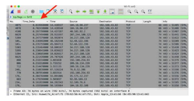
Remove the previous filter from the filter toolbar and again double-click the Time\_Delta header column to sort the time delta values. This enables you to see the major delays between packets in each separate TCP stream, which is useful for considering and deciding which stream do you want to troubleshoot and which one you don't, as shown in the figure below.
