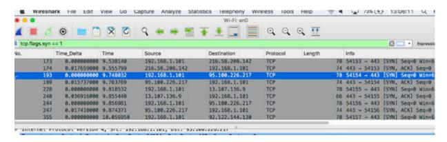
In the Packet List pane, select a SYN packet. In the Packet Details pane, click the Flags field to open the tree view and verify the flags related to the window size, as shown in the figure below (where the Reduced Window is not implemented).
