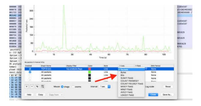
In the figure above, the green graph shows all packets because no display filters have been applied. Therefore, all traffic seen in the trace file has been graphed, that is, the entire size of all packets (including headers and data).
