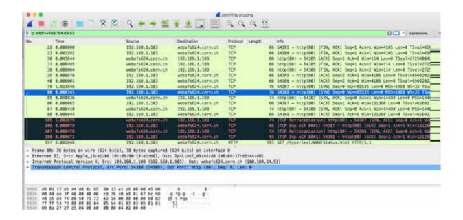
By default, Wireshark is configured to dissect HTTP on the following ten ports: 80, 3128, 3132, 5985, 8080, 8088, 11371, 1900, 2869, and 2710. However, other ports can also be used for HTTP communication. You can specify the ports in the Preferences dialog box. On the main menu, select Edit > Preferences. In the left tree view, select HTTP and then enter the ports in the TCP port(s) box.
