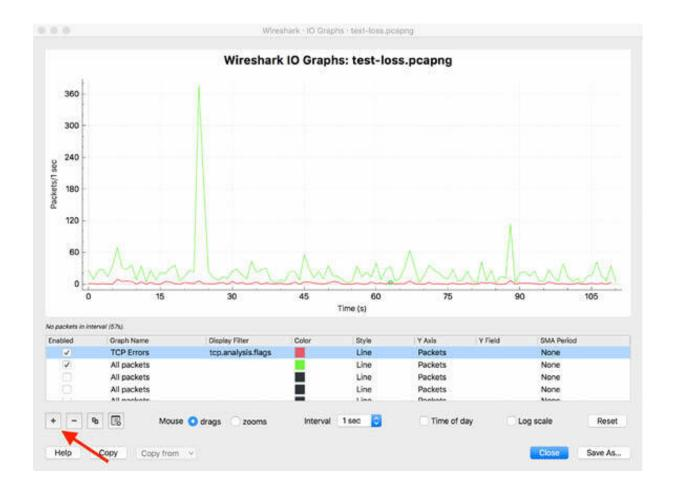
You can also alter the X axis to change the tick interval and the pixels per tick. In the Interval list, change the tick interval.
