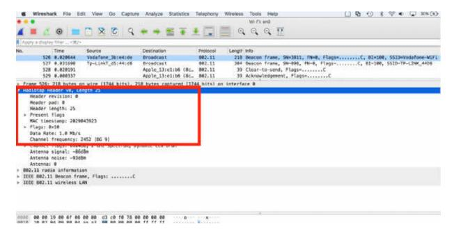
Repeat the same steps by selecting the PPI Header. Alternatively, you can download the sample capture file mesh.pcap from <a href="https://wiki.wireshark.org/SampleCaptures">https://wiki.wireshark.org/SampleCaptures</a> . The resultant window will look as shown in the figure below.
