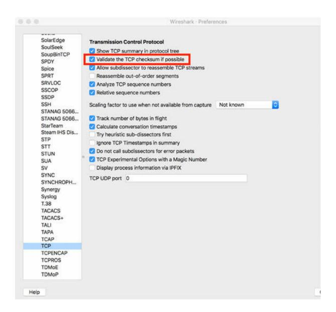
If you are capturing trace files on your own system and each TCP packet sent from your host indicates that the TCP checksum is invalid, your network interface card and the driver may support checksum offloading. You can also disable the Checksum Errors coloring rule or specific checksum validation processes.
