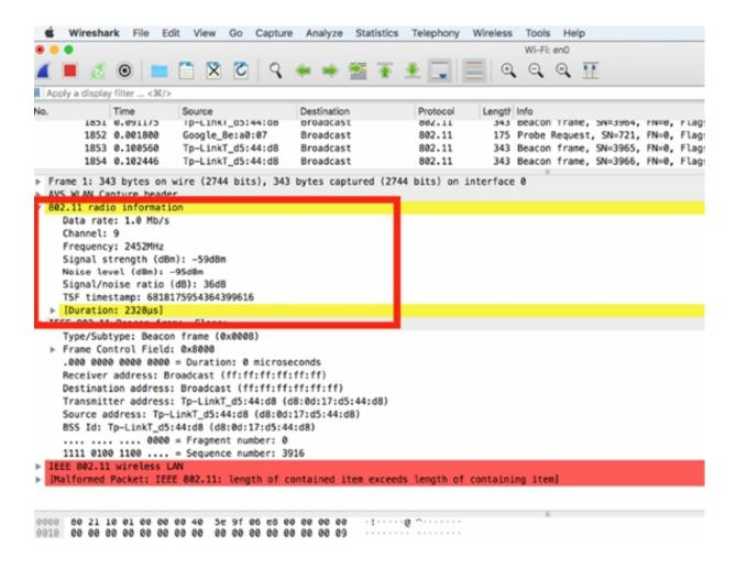
To filter the 802.11 frequency/channel information, apply the radiotap or PPI header. This information is not sent with a packet as a field value. When the adapter receives the WLAN packet, the frequency that the packet was captured on is used to define which channel the packet was on. This frequency/channel information is shown in the radiotap and PPI headers.
