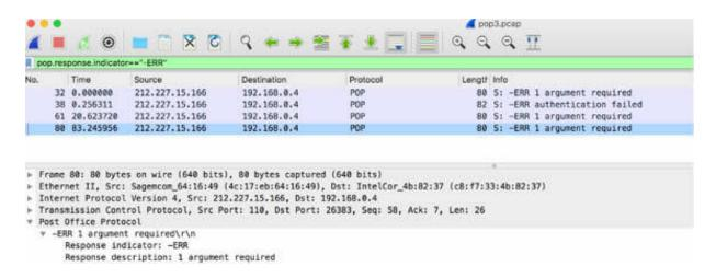
To display only a specific request command (for example, RETR), in the filter toolbar, enter pop.request.command=""RETR", as shown in the figure below.
