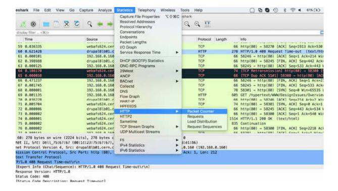
The Packet Counter dialog box is displayed listing the Status Code responses. When analyzing HTTP communication, this information is useful because it makes it easy to spot 4xx Client Error or 5xx Server Error responses, as shown in the figure below.
