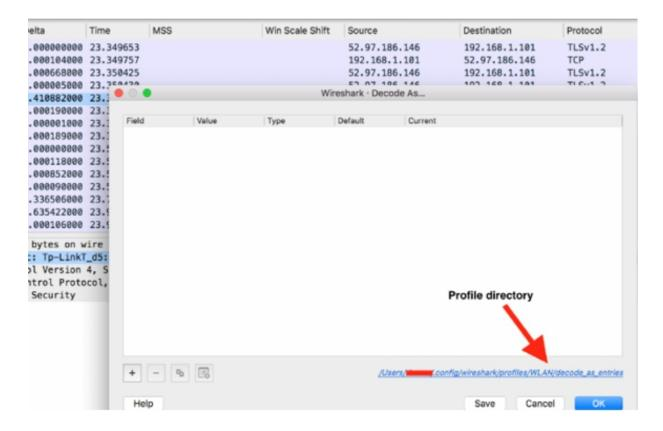
You can also define preferences for some applications, such as HTTP, and configure Wireshark to recognize additional or alternate port numbers for applications. On the main menu, click Edit > Preferences. In the
