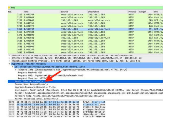
If no port number is specified, the default port for the service (for example, port 80 for HTTP) is used.
