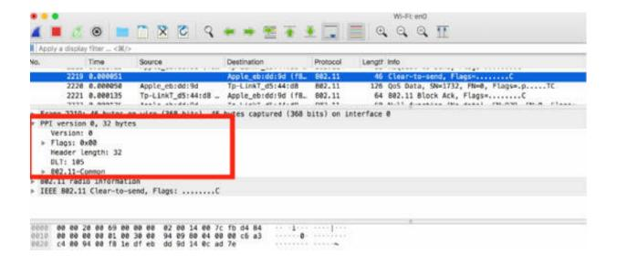
From the previous two figures, it is clear that the radiotap and PPI headers supply additional information about the frames captured. The radiotap header provides this information from the AirPcap or libpcap driver to Wireshark, because it is not in the WLAN packet when it arrives, it is added by the local capture adapter.
