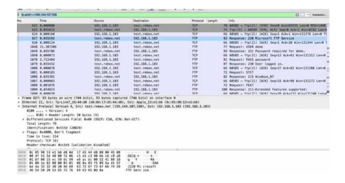
In the figure above, as shown in packets #622, #623, and #624, an FTP connection begins with a TCP handshake followed by the client waiting for the banner.
