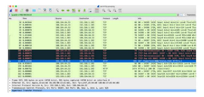
As shown in the figure below, the client made a three-way TCP handshake from port 54388 to port 80. In the Info column, packets #80, #85, and #86 are listed as HTTP because transport name resolution is enabled.
