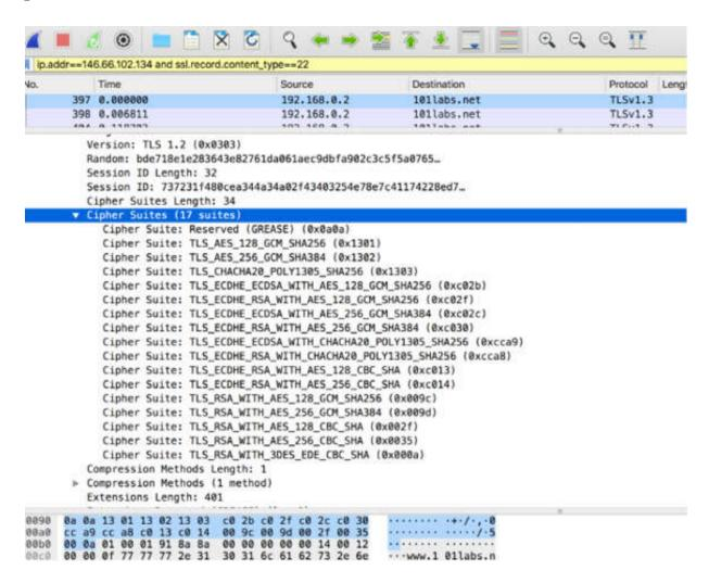
At the end of the TLS packet, after the "Compression Methods" field, there are a series of extensions. These extensions add functionality to TLS.
