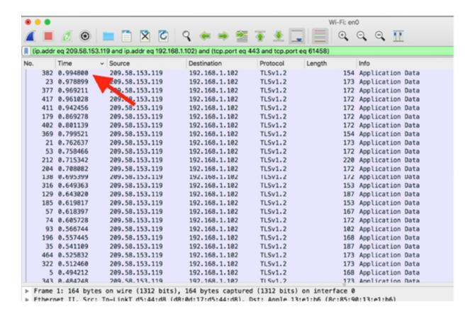
You can also add a new column by using the Preference dialog box, where you can select an additional delta time. Another option is to inspect the packet content in the Packet Details pane, as shown in the figure below.
