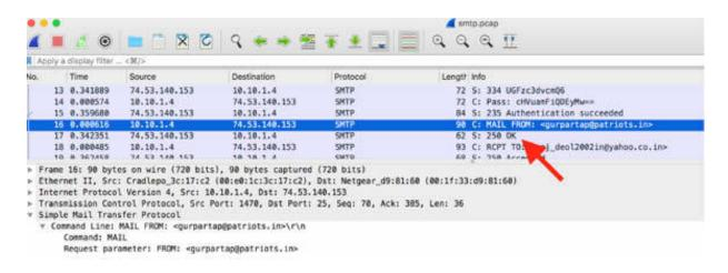
The client sends the RCPT TO message with the next packet, indicating to whom the email will be sent (packet #18), as shown in the figure below.
