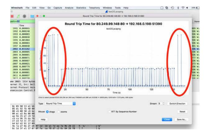
Vertical stripes can happen when the packet loss occurs and a high number of duplicate ACKs are sent. Another scenario for vertical stripes is when data is queued along a path, and then it is suddenly forwarded through the queuing device.
