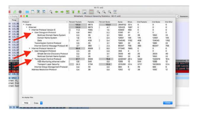
When baselining such types of traffic, you need to identify which applications are running on the network and which protocols are being used. If the applications use TCP, identify the TCP ports. Similarly, for UDP ports, identify the UDP ports.
