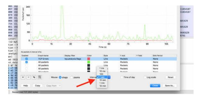
You can also adjust the Y axis to correctly set the units and scale. Double-click the "Y Axis" field to select a unit.
