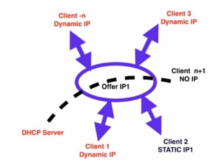
In the network, "Client 2" exists with a static IP1, while all other clients have dynamic IP. When "Client n+1" enters the network, the DHCP server offers the exact IP1 to the new client. The DHCP client can perform the duplicate address test. If the DHCP client locates another host with the same address, it must decline the IP address provided in the DHCP offer. It, however, remains with no IP address assigned.
