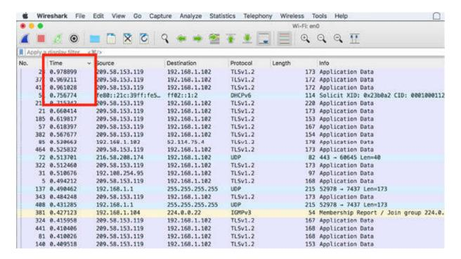
If the capture file contains numerous conversations, then before sorting the Time column, filter a conversation to ensure that you are comparing times within a single conversation. To do so, on the main menu, select Analyze > Conversation Filter, as shown in the figure below.
