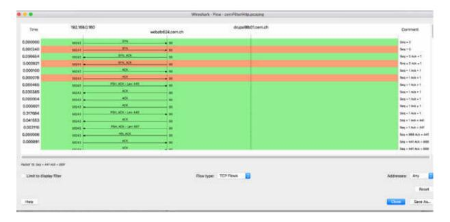
You can also choose a node address type. Choose standard source/destination addresses when many hosts are communicating with each other, and you need to narrow the output. This option shows the IP addresses of devices listed in the graph. Choose network source/destination addresses when you are using network name resolution with Wireshark.
