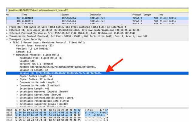
The client provides the list of cipher suites (inside the "Cipher Suites" field) supported by the browser. In this case, the client supports 17 cipher suites and lists them all in the "Client Hello" packet. In the end, the server decides which cipher suite to use, but the cipher listed at the top is the client's preference.
