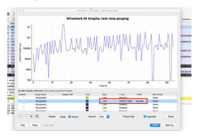
In this example, there are two unusual drops around 100s and 110s. If you click on the graph at that specific point, you can jump to the packet in the Packet List pane and inspect whether a problem occurred in the data transfer.
