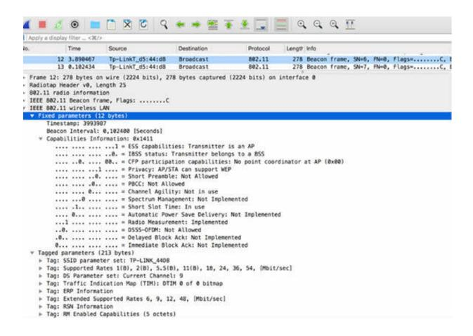
In the figure above, packet #12 is a beacon frame with the "Capabilities Information" field expanded in the Packet Details pane. Based on the "ESS Capabilities" field shown in the figure below, it is clear that the transmitter is an access point (AP).
