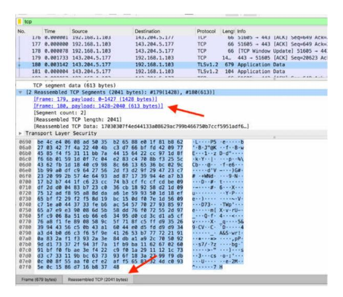
To get the Packet Details data reassembled or view a frame split in non-reassembled format, click the "Reassembled TCP" tab, shown in the figure above.
