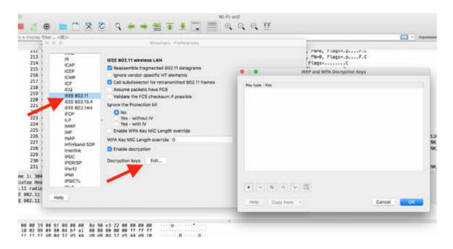
Wireshark can decrypt WEP, WPA, and WPA2 traffic. When decrypting WPA traffic, you must capture the four EAPOL (Extensible Authorization Protocol) four-way handshake packets.
