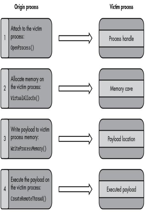
Figure 12-5: Basic process injection
