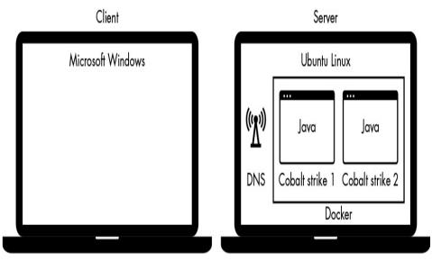
Figure 5-1: The lab setup for creating your DNS server
