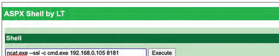
Figure 5.16: Uploading and executing the ncat.exe command on the server via a web shell
