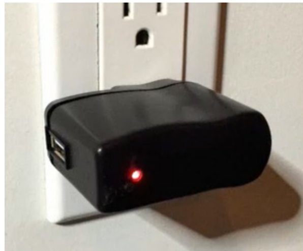
Figure 7.7 – A keylogger hidden inside a USB charger
