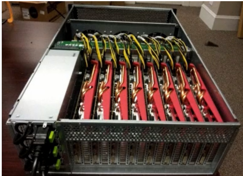
Figure 7.8 – GPU cracking system
