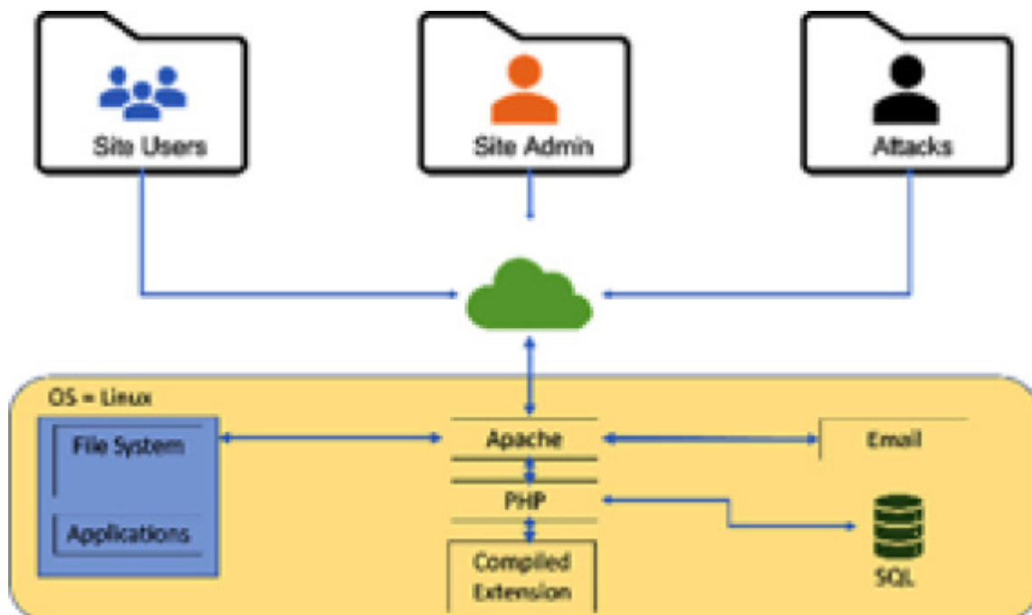
Figure 13.1 – A typical open source architecture for a web server and its applications
