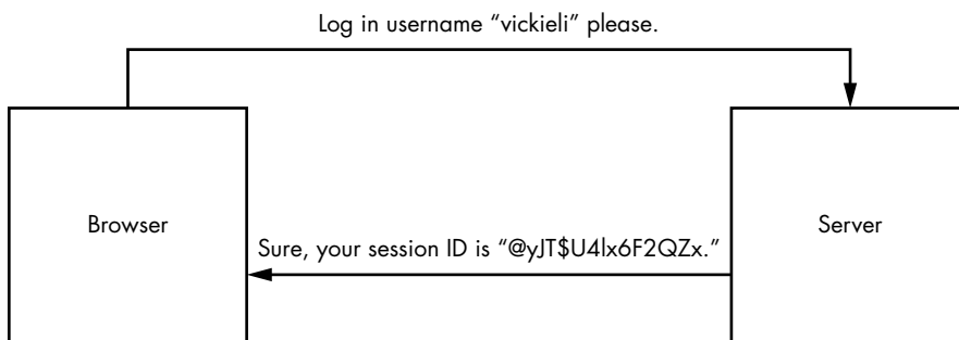
Figure 3-4: After you log in, the server creates a session for you and issues a session ID, which uniquely identifies a session.
