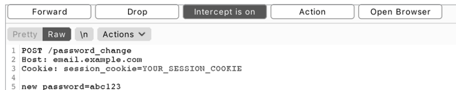
Figure 9-3: Set to Intercept is on to capture your browser's traffic. Click the Forward button to forward the current request to the server.
