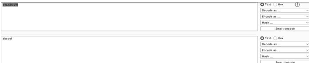
Figure 10-2: You can try to use different methods to decode a string in Burp's decoder. Or you can use the Smart Decode tool and see if Burp can detect the encoding scheme.
