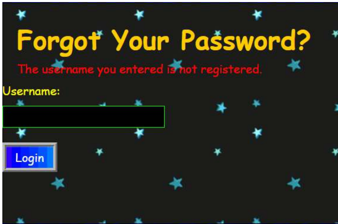
Figure 9.13: Checking username enumeration with nonexistent username
