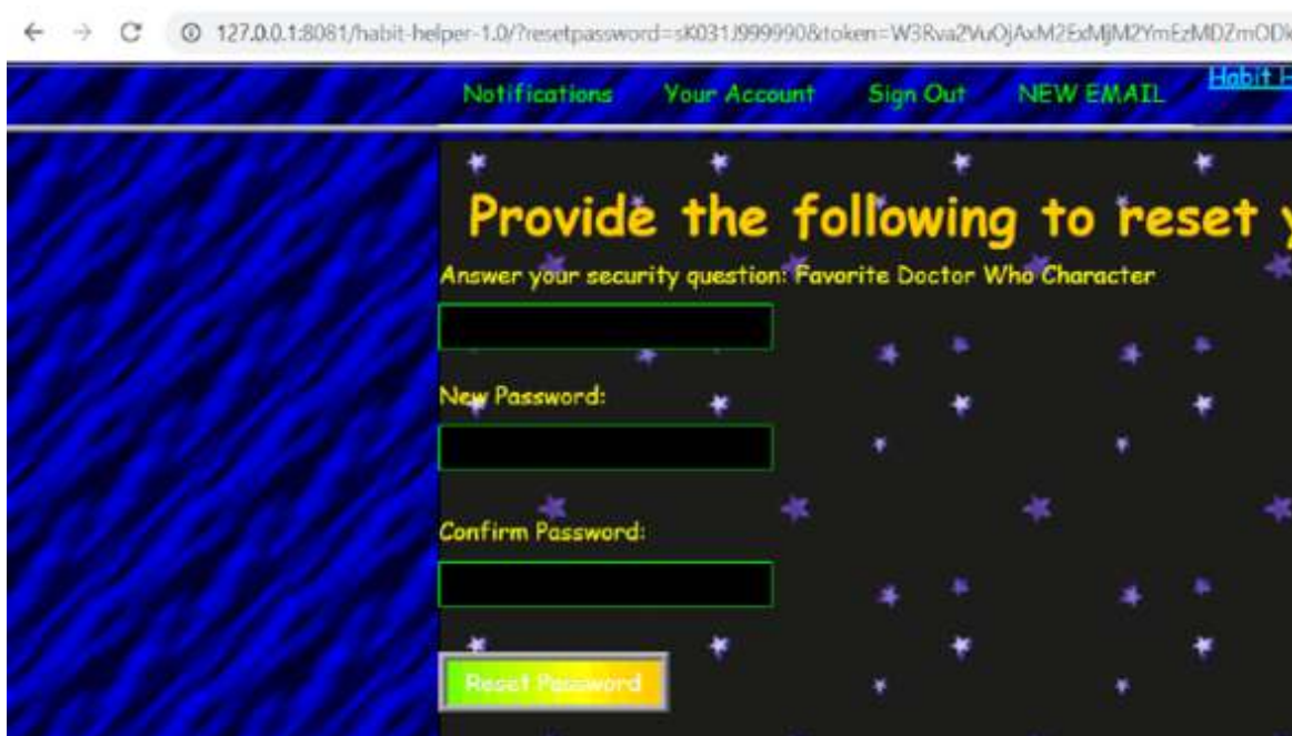
Figure 9.31: Security question changed with manipulation of resetpassword parameter
