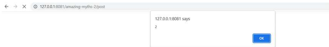
Figure 6.14: Client-side bypass cross-site scripting execution
