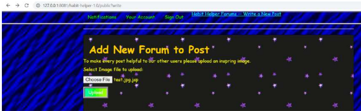
Figure 8.14: Try to upload a double file extension
