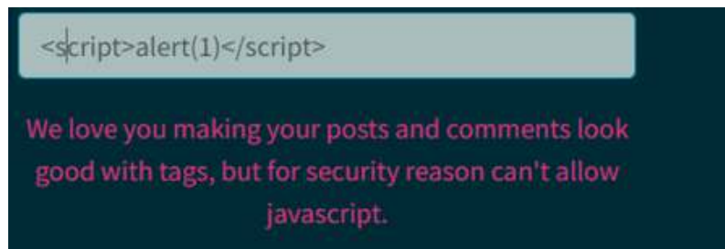
Figure 4.28: Using script tag to test for XSS
