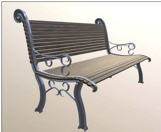
FIGURE 7-1: With the exception of the slats for the seat and back, this entire park bench was modeled with curves.
