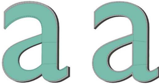
FIGURE 5-3: Insetting (right) creates a nicer border on a complex shape than just extruding and scaling (left).
