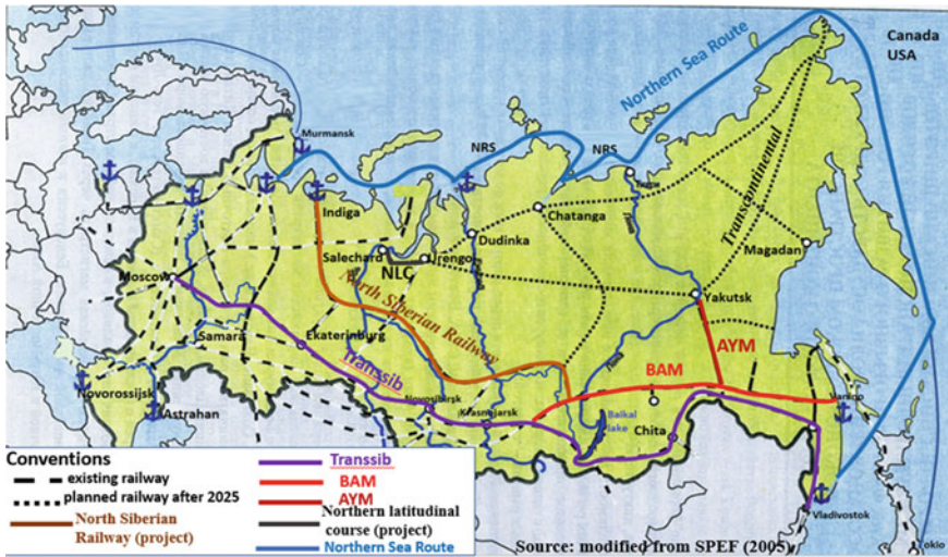
Fig. 1 Overview scheme of the primary transport railway network leading directions in Russia in the first quarter of the twenty-first century and planned schemes
