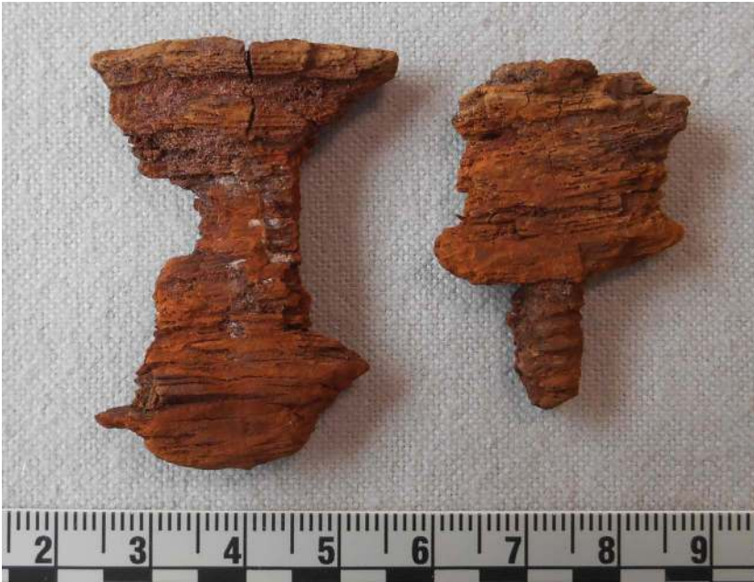
Figure 5.35 Examples of highly corroded iron screws surrounded by remnant portions of coffin wood; historical context, Massachusetts, USA. The iron oxide has helped preserve the surrounding wood. The scale is in cm.
