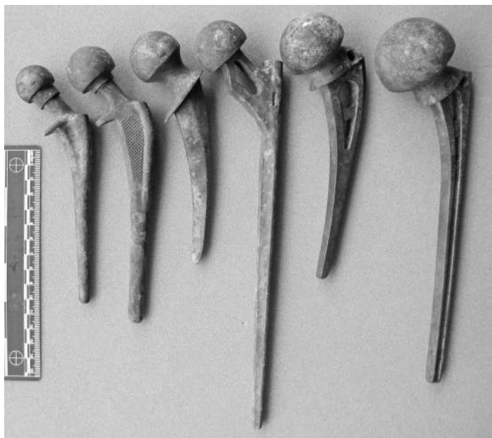
Figure 14.4 Surgical implants (titanium alloy femur head replacements), all of which have survived commercial cremation in excellent condition. The scale is in cm. (Photographed materials courtesy of Ranald Donaldson, University of Victoria, Saanich, BC, Canada.)
