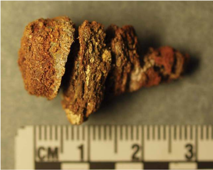
Figure 5.32 Example of a highly corroded screw surrounded by remnant portions of coffin wood; historical context, Massachusetts, USA. The screw head is to the left. The metal oxides have helped preserve the surrounding wood. The scale is in cm.
