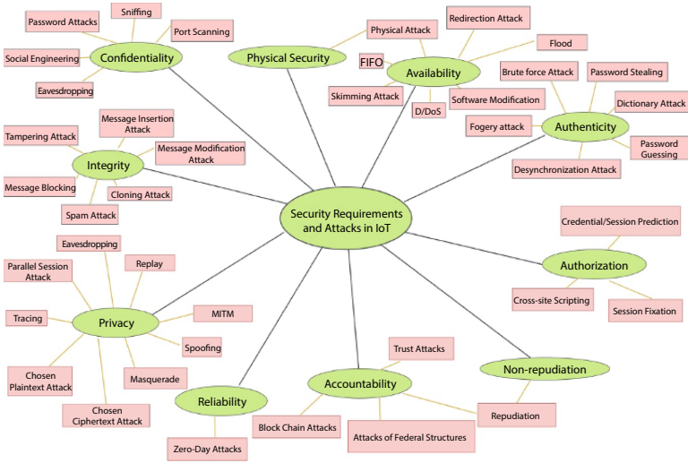
Figure 1.2 Security requirements and attacks in IoT.
