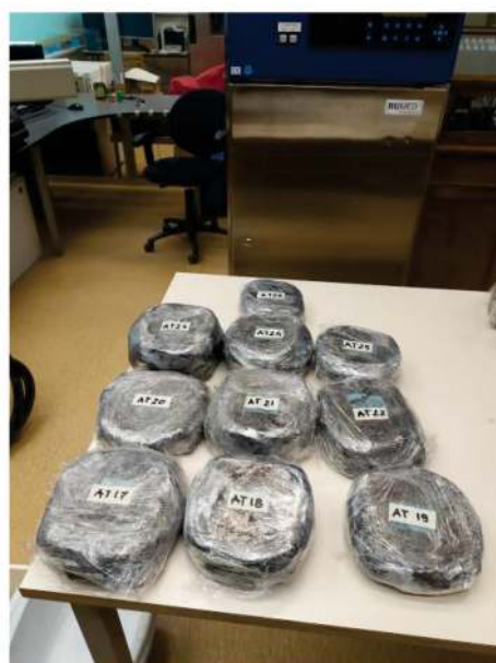
Figure 6. Preparation of specimens for the oedometer tests.
