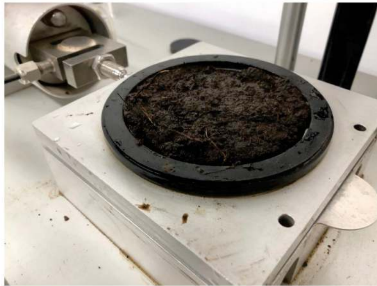
Figure 5. Placement of the test specimen in the Eijkelkamp displacement apparatus.
