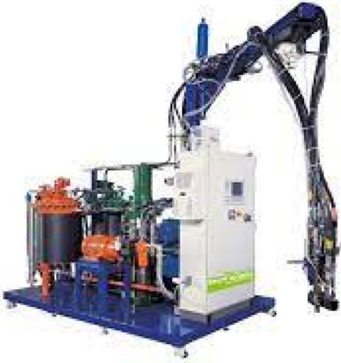
Figure 11.8 Polyurethane metering machine for foam. Source: PUR foam (2020).
