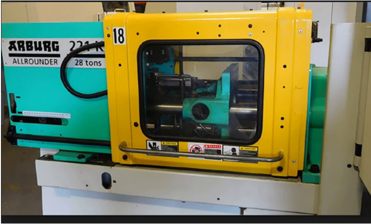
Figure 13.17 Arburg 25 ton injection molding machine at California State University, Chico.
