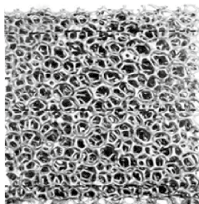
Figure 9.27 Open (b) and closed (a) cell foam structures. Source: Foam (2020).
