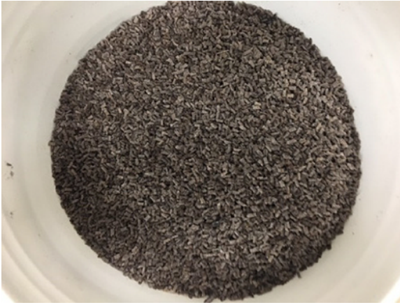
Figure 13.15 Plastic pellets of almond shell powder blended with recycled polypropylene plastic and extruded in a twin-screw extruder. These pellets can be injection molded in an injection molding machine to make parts.
