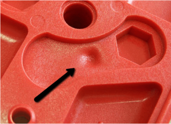
Figure 14.10 Sink marks in plastic molded parts. Source: Sink marks (2020).
