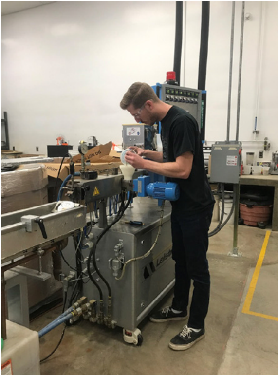
Figure 13.18 Students working on the twin-screw machine adding almond shells. Source: Permission granted from Mr. Marshall Ellis.
