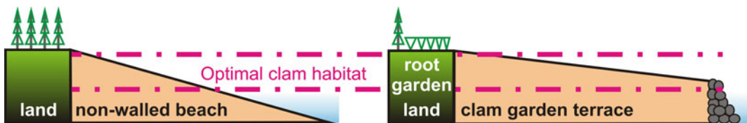
Fig. 3.1 Sectional schematic illustrating the basic architecture of a clam garden. The structure of the clam garden (at right) is compared with the profile of the original beach (at left). Clam gardens were often accompanied on the landward side by root gardens, which were tended for a
