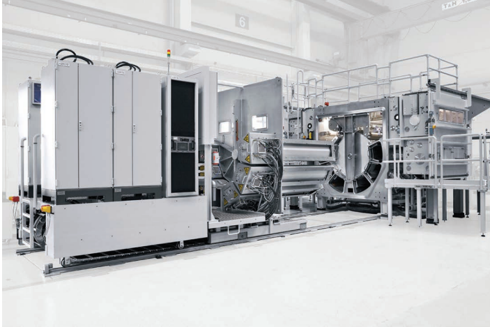
FIGURE 7.2 APPLIED SMARTWEB® roll-to-roll sputter coater for ITO and other conductors, by permission of Applied Materials Inc.
