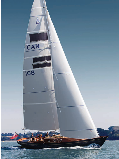
FIGURE 8.4 Solar sail on the sailing boat, Spirit 44CR(e). (Photograph by Richard Langdon, courtesy of Solar Cloth, France.)
