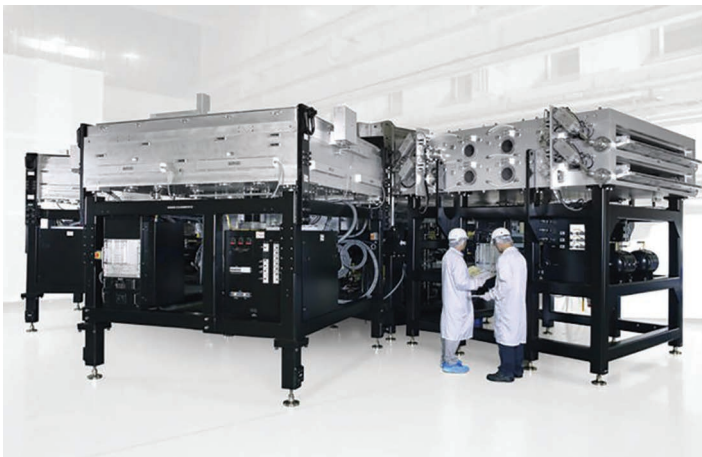
FIGURE 7.1 Large-area PECVD amorphous silicon coater for liquid crystal displays, by permission of Applied Materials Inc.
