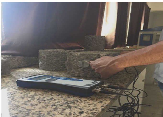
Fig. 4 Ultrasonic pulse velocity test
