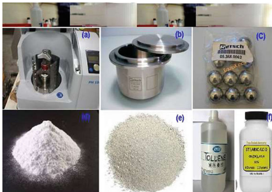
Fig. 4 Initially all the materials required for experiment were made ready in the material testing laboratory. a Retsch PM 100 ball mill used for mixing as well as milling. b Hard stainless steel jar used to hold hard steel ball that helps/milled the material under processes. c Hard stainless steel ball that was used with Jar, d ceramics powder, i.e. Al_2O_3 e Aluminium powder used here as base material for composite. f Liquid toluene was used as a solvent and stearic acid as lubricant used in the material preparation method
