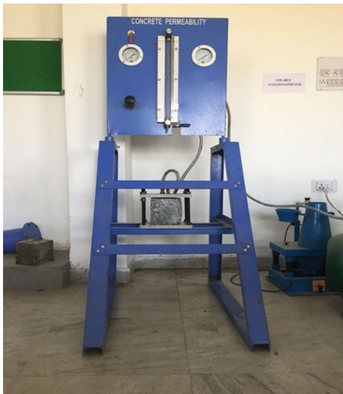
Fig. 3 Water permeability test
