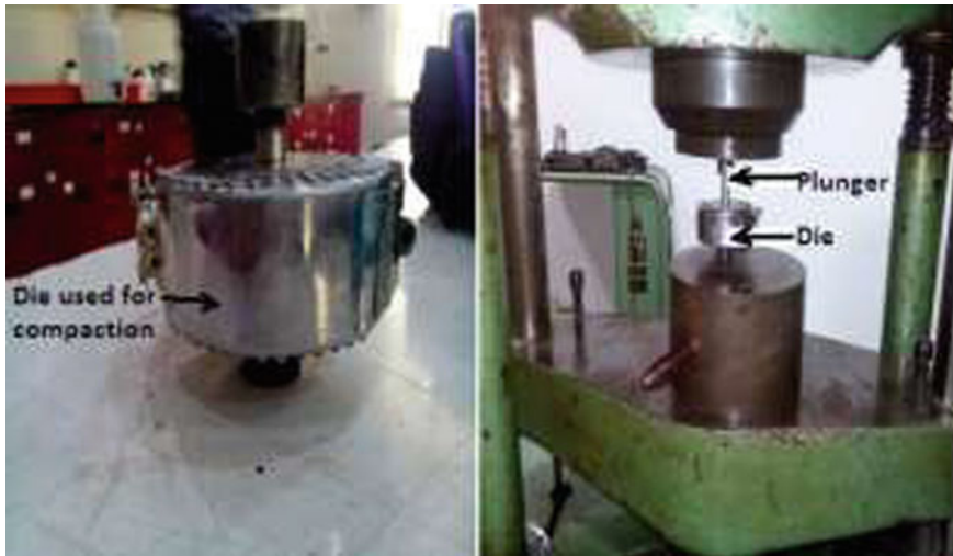
Fig. 5 Die and plunger used for compaction
