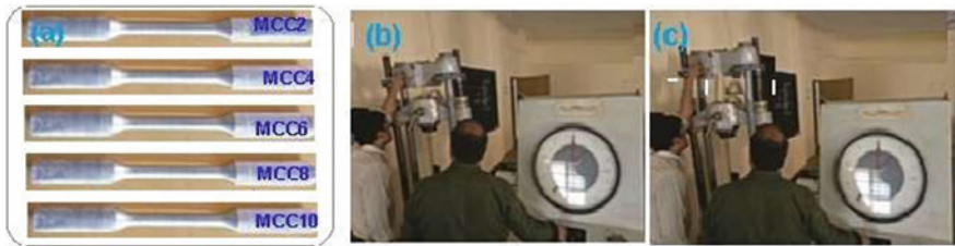
Fig. 10 a Five different test samples used for tensile test, b initial setting of sample in UTM has been done and c the final elongation of sample
