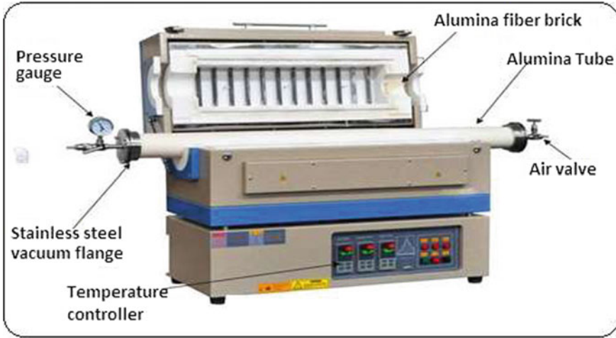
Fig. 6 High temperature tubular furnace and its different subassemblies kept in material testing laboratory in IIT, Roorkee
