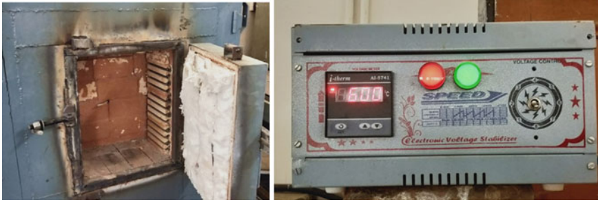
Fig. 2 Electric furnace with control panel
